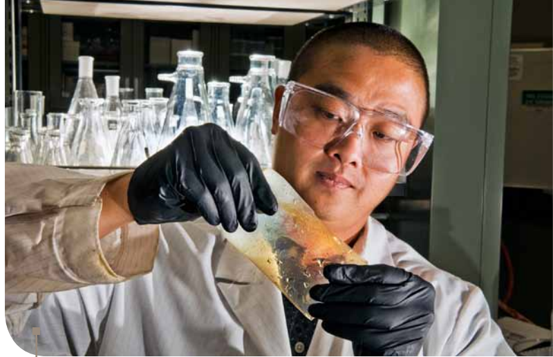
Sandia researcher Cy Fujimoto demonstrates his new flexible hydrocarbon polymer electrolyte membrane, which could be a key factor in realizing a hydrogen car.
