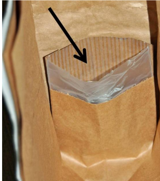
Figure 6.6. Extended polyethylene bag valve, interior view.
