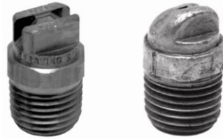
Figure 2.19. Nozzle damage—new versus used [SSCO 2003].
