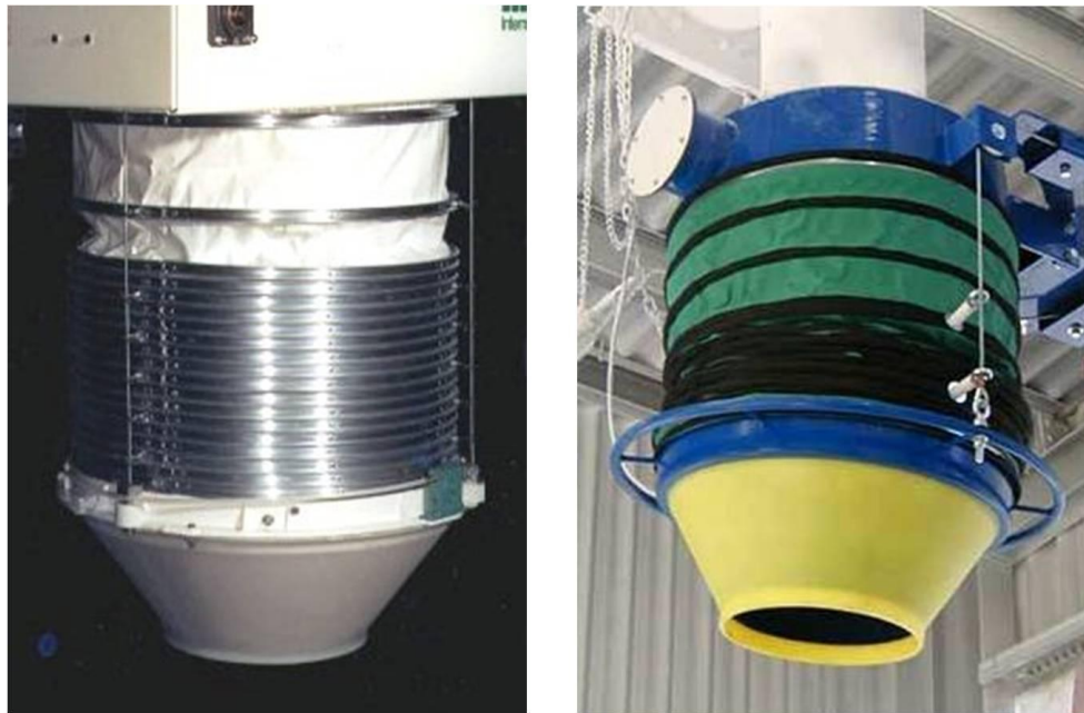
Figure 7.2. Loading spout discharge cones designed to seal against the loading port of closed vehicles to minimize dust liberation.
