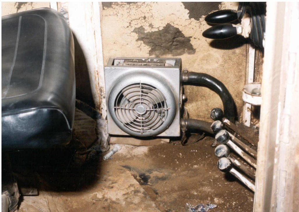
Figure 8.13. Product tracked onto the floor of a piece of mobile equipment from dirty work boots.
