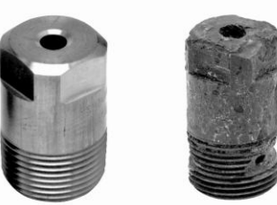
Figure 2.18. Temperature damage—new versus used [SSCO 2004].
