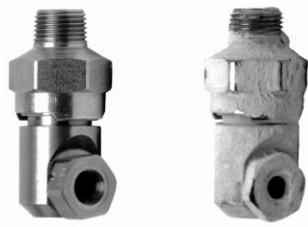
Figure 2.17. Nozzle caking—new versus used [Schick 2006].
