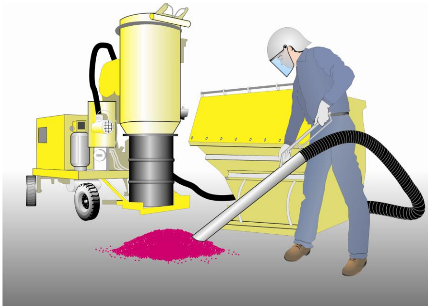
Figure 8.6. Portable system used to perform vacuuming.
