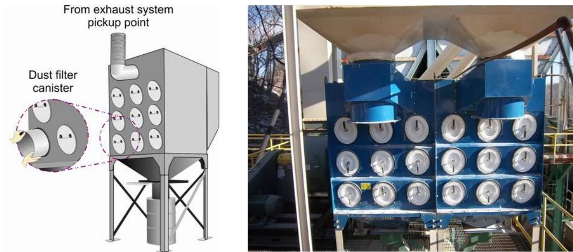
Figure 1.20. Cartridge collector with dust filter canisters.
