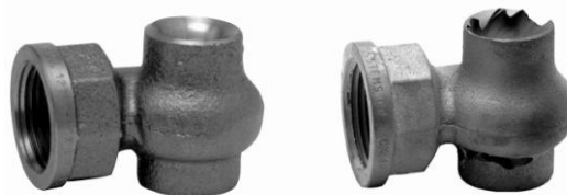
Figure 2.15. Nozzle erosion—new versus used [Schick 2006].
