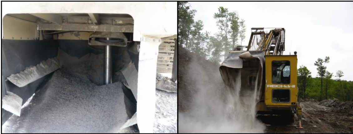
Figure 3.11. Buildup of material on the air-blocking shelf (left) and the resulting dust emissions that are created during lowering of the drill mast (right).
