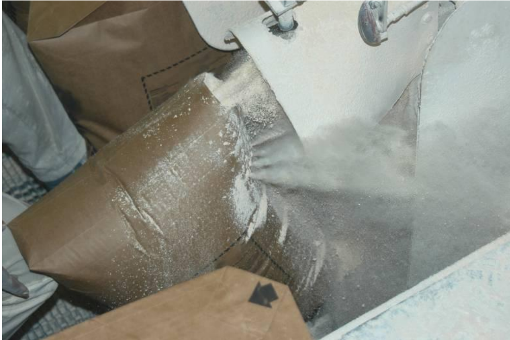
Figure 6.4. Undervalue perforations relieve excess pressure from bag during filling process to minimize the possibility of bag failure. Product and dust are seen escaping along with excess air.
