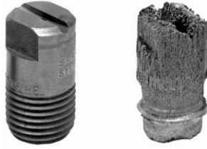
Figure 2.16. Nozzle corrosion—new versus used [Schick 2006].
