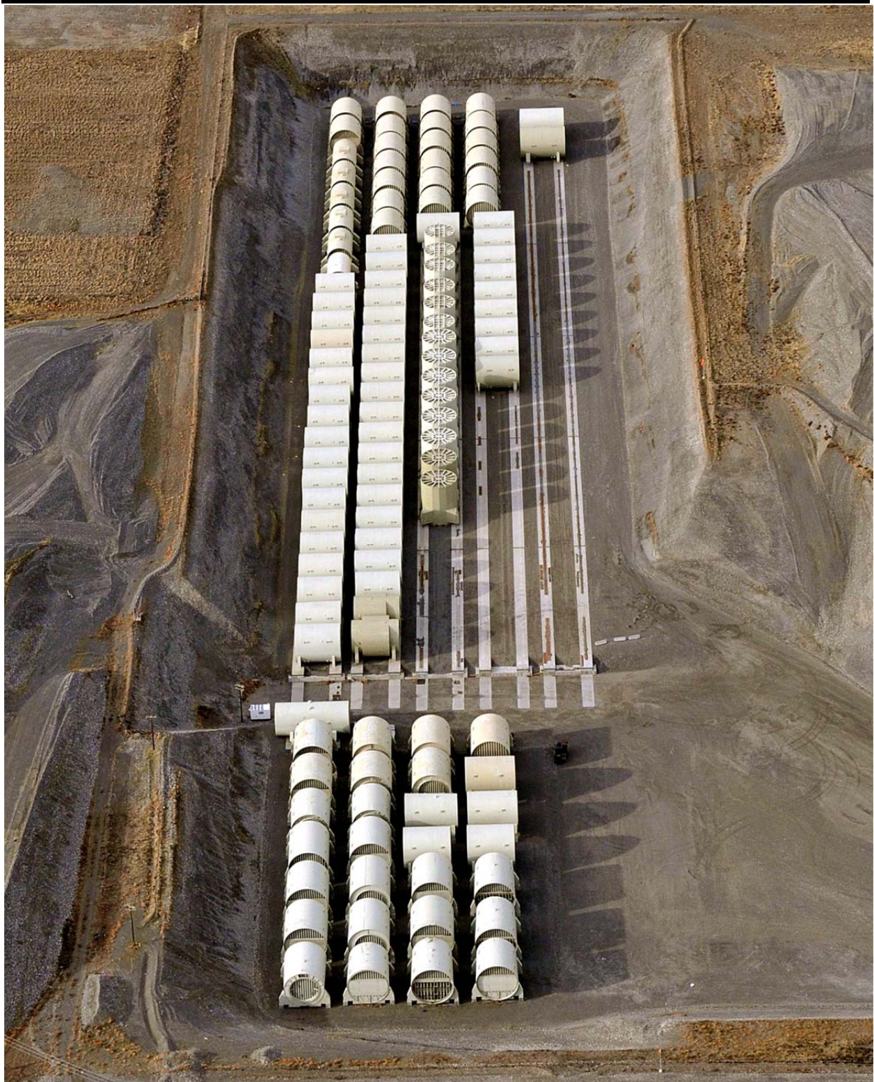
Figure 2.6. Pre-LOS ANGELES Class, LOS-ANGELES Class, and Cruiser Reactor Compartments in Trench 94, November 2009
