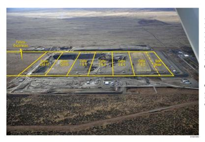
Expansion of Hanford's Environmental Restoration Facility is made possible with funding from the American Recovery and Reinvestment Act. Construction of super cells 9 and 10 will increase waste disposal capacity of the facility by 50 percent and will be completed in September 2011.
