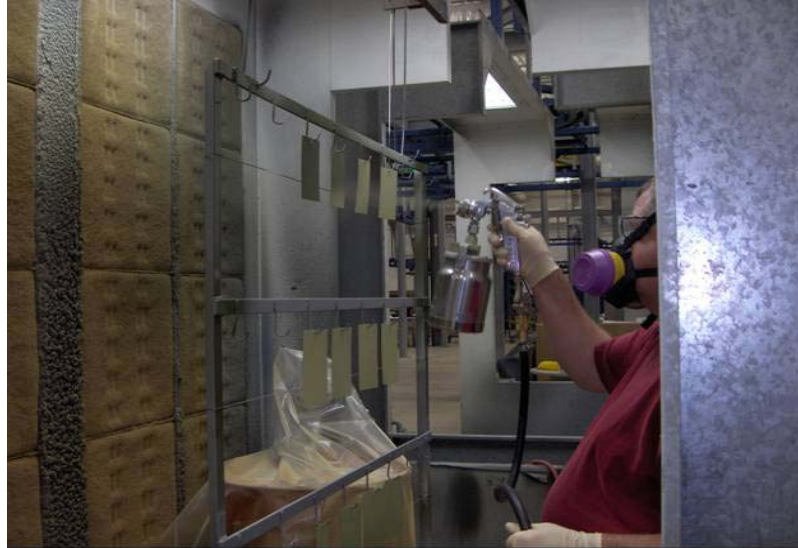
Figure 3: Wet Spray Application at CTC
