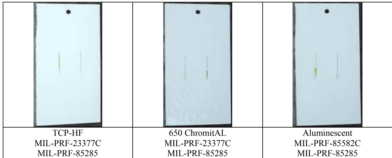
Figure 5: Representative Photos of Trace Adhesion Loss
