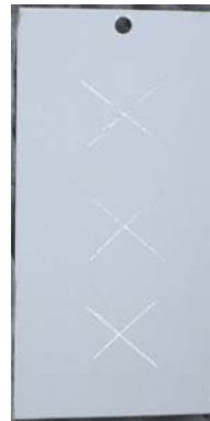
Figure 9: Dry Tape Adhesion Test Panel
