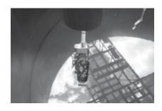
This photo, taken at Hanford's Cold Test facility, shows the tank crawler being lowered into the tank using robotics. Operators can test the equipment, and learn how to use it with this safe mock-up of a tank.
