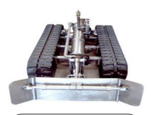
This tank crawler was designed to be lowered into Hanford tanks to assist in retrieving waste. The bulldozer-type blade on the front can push waste toward vacuum equipment.
