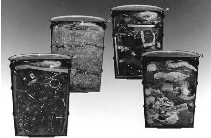
Drums of waste, simulated examples shown here, are x-rayed at the Waste Receiving and Processing Facility as part of the process to prepare them for shipment offsite.
