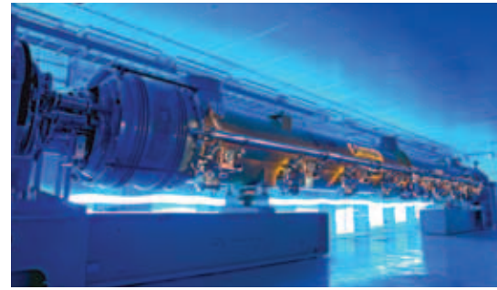
Left: Composed of eight 9-cell superconducting radio-frequency cavities arranged end to end and nestled in a long tube to keep them cooled to temperatures near absolute zero, the cryomodule at Fermilab is the only one of its kind in the United States.
