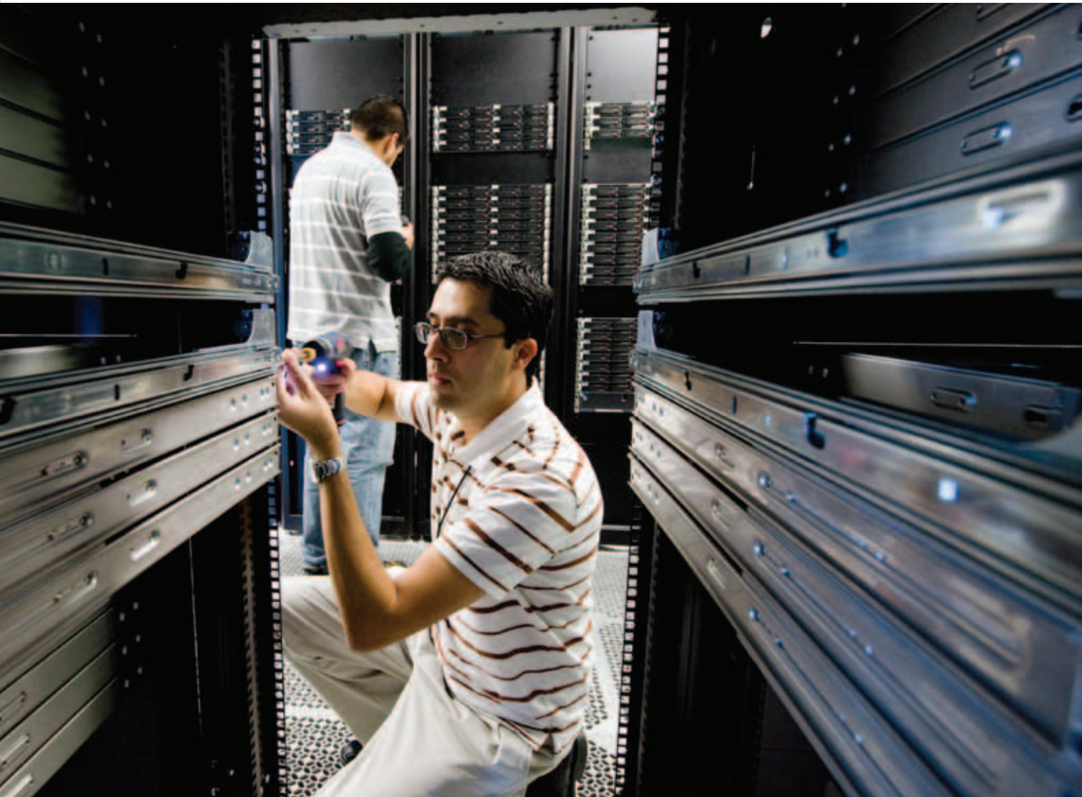
Above: Fermilab scientist Don Holmgren performs maintenance on a GPU, or graphics processing unit, computer. Scientists have begun to exploit GPUs for the ability to do parallel computations with very high efficiency and low power consumption.
