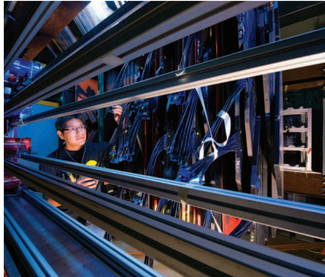
Above: The MINERvA detector is located in an experimental hall 350 feet underground. Scientists can install various targets to investigate how neutrinos interact with different types of nuclei.
