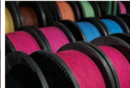
Left: Electron beam treatment improves the heat resistance of coatings for wire and cable by crosslinking the polymers in the material.
