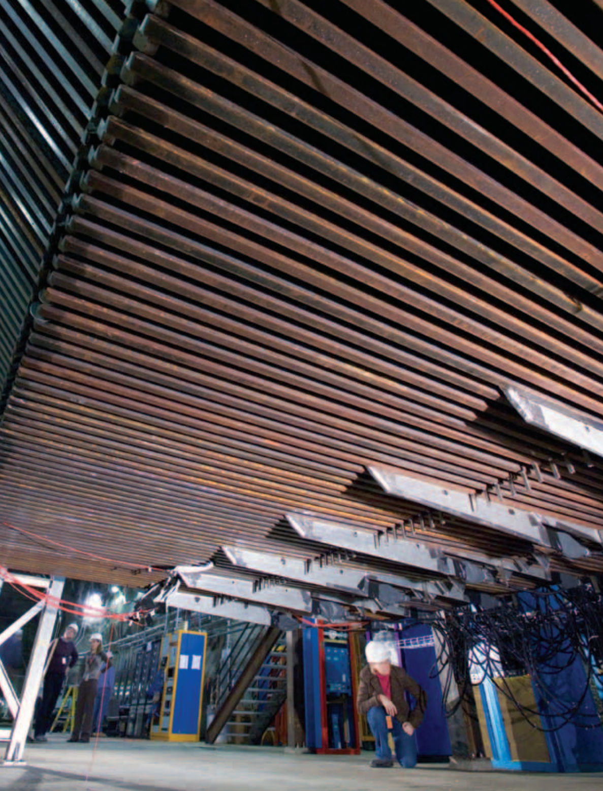
Above: The MINOS near detector, located 350-feet underground on the Fermilab site, checks the purity of a muon neutrino beam as it leaves the Fermilab site.
