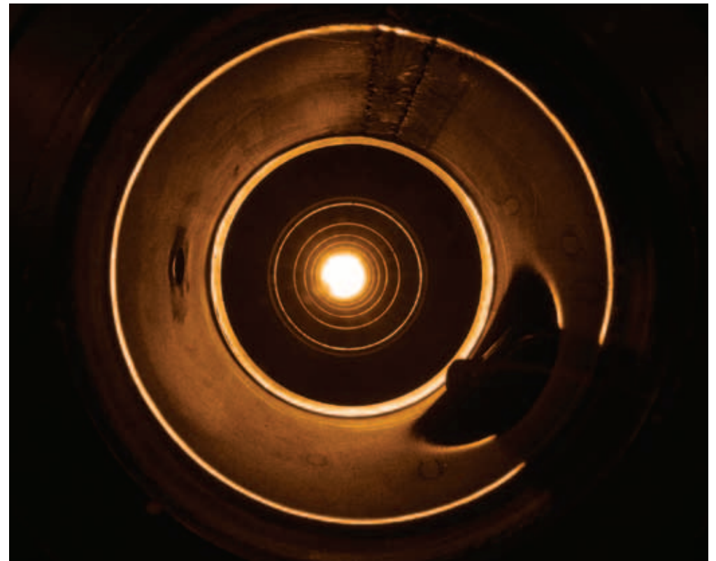
Below: A superconducting radio-frequency cavity from the viewpoint of a positron or electron beam. The cavity kicks the beams to higher energies, preparing them for collision.
