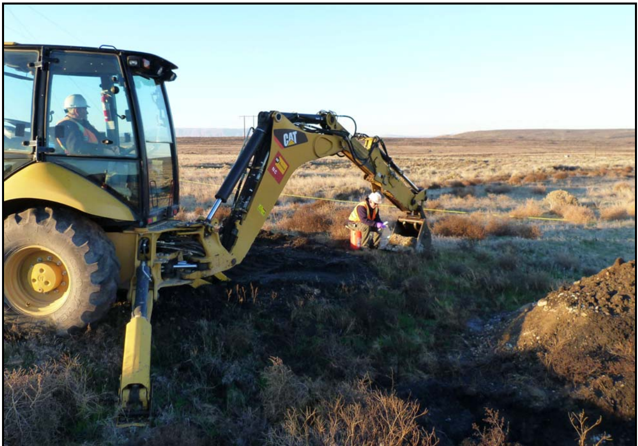
Washington Closure Hanford subcontractor TerranearPMC conducts confirmatory sampling activities at 600-323. The site consists of the underlying soil and a bermed area with coal cinders. (Photo 10)
