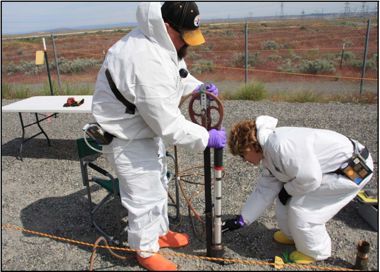
Washington Closure Hanford subcontractor North Wind used a multi-detector probe to characterize one of 50 vertical pipe units at the 618-11 Burial Ground. (Photo 6)
