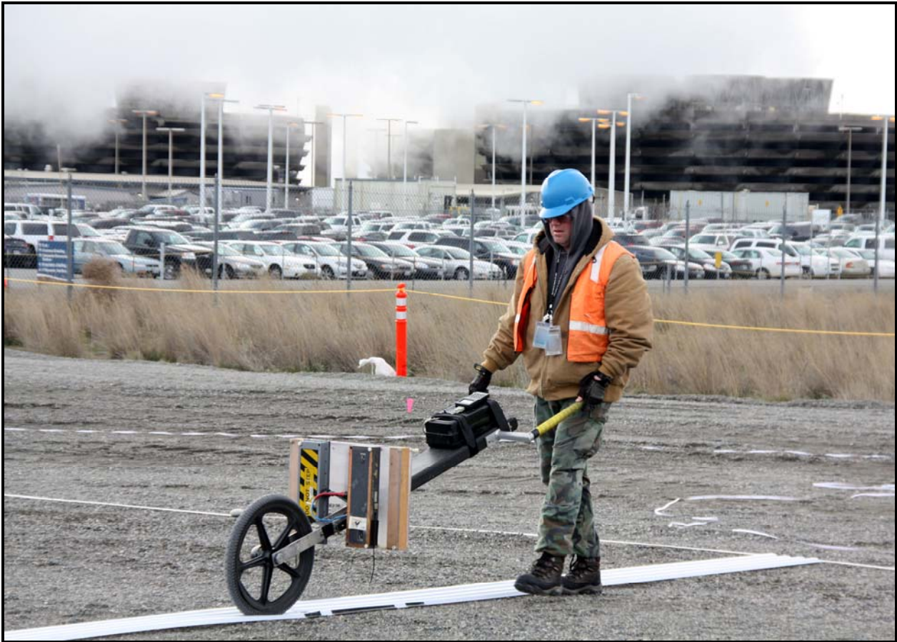
Washington Closure Hanford subcontractor Sage Earth Science of Idaho Falls, Idaho, performs geophysical delineation at the 618-11 Burial Ground. (Photo 3)
