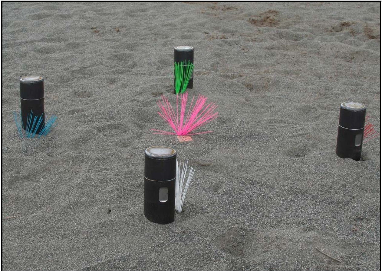
Four cone penetrometers are installed around each of the 94 vertical pipe units at the 618-10 Burial Ground.
