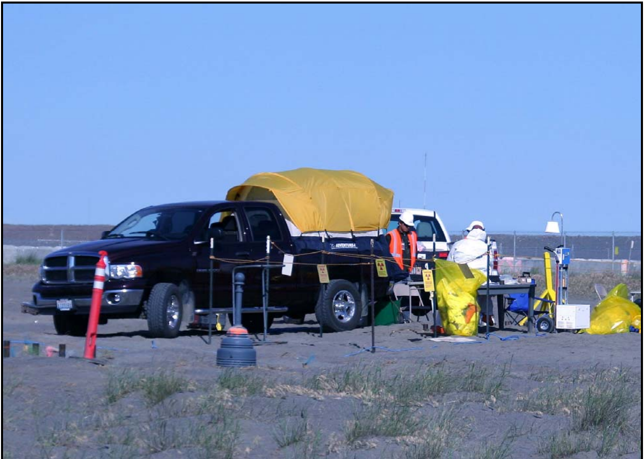
Nonintrusive characterization activities concluded at the 618-10 Burial Ground. Measurements were collected for 100 cone penetrometers in the trenches and 376 in the vertical pipe unit area.
