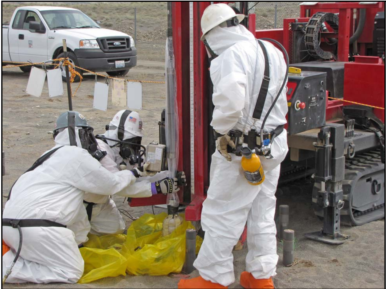
Workers collect a soil sample as it is retrieved from a cone penetrometer during soil sampling activities at the 618-10 Burial Ground.
