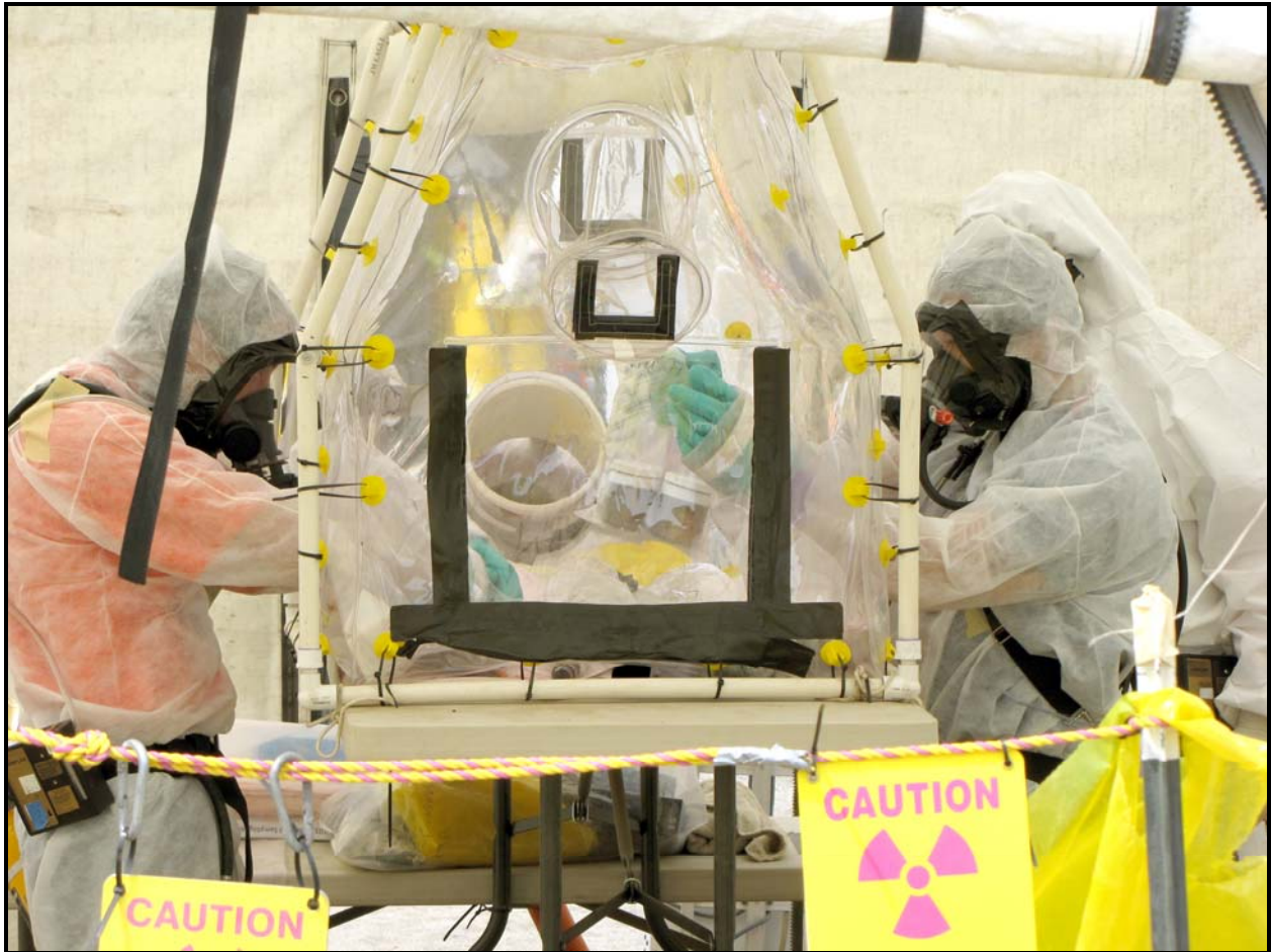
Workers transfer a soil sample to a sample bottle inside a table-mounted glovebag during soil sampling activities at the 618-10 Burial Ground.
