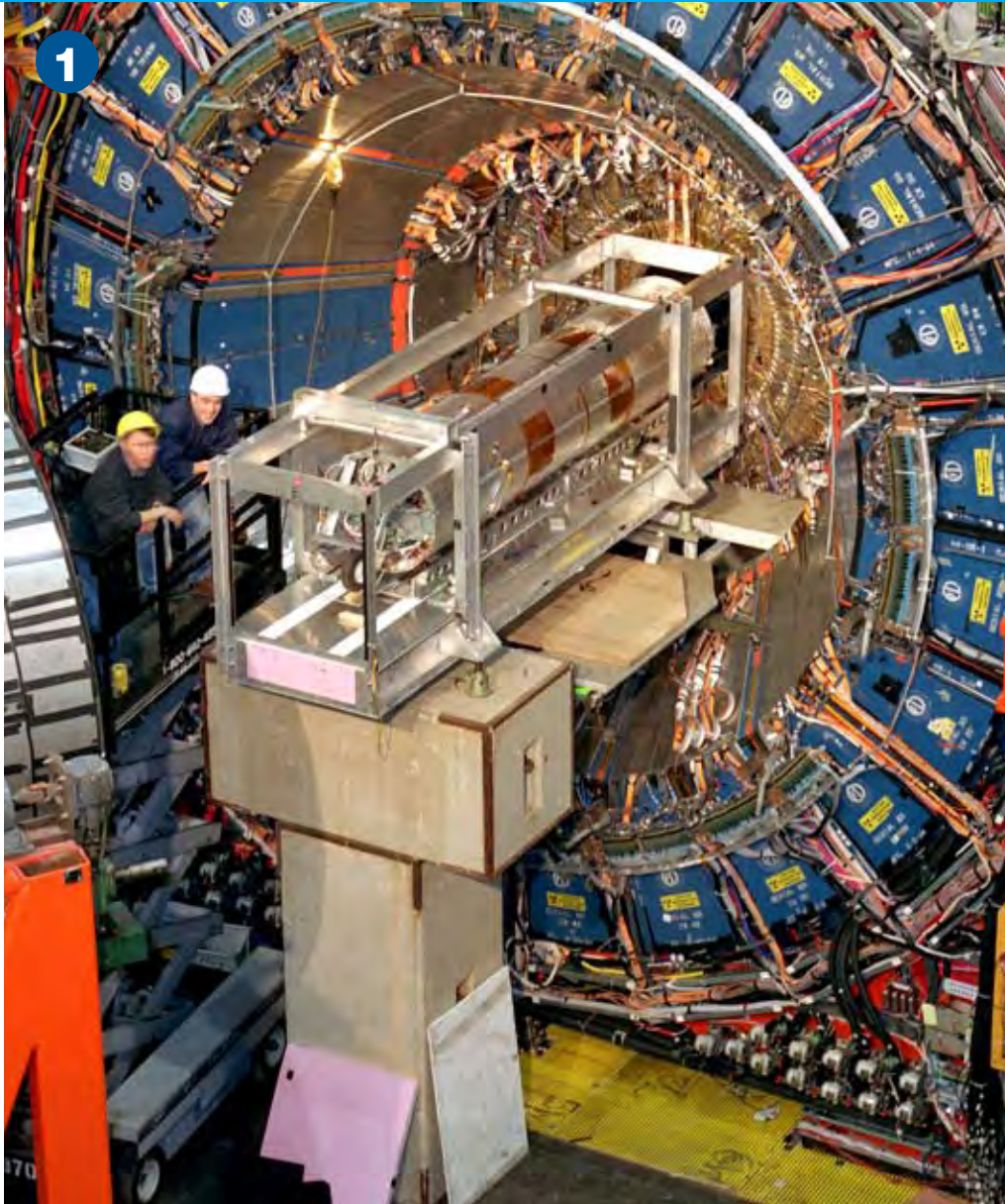
1 The roughly 6,000-ton CDF detector comprises layers of subdetectors that surround the particle collision area, like layers of an onion.
