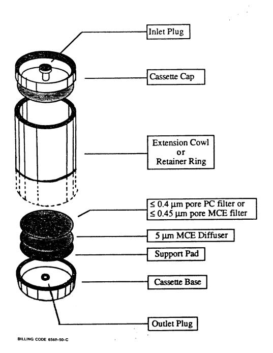
h. When polycarbonate filters are used, position the highly reflective face such that the incoming particulate is received on this surface.
