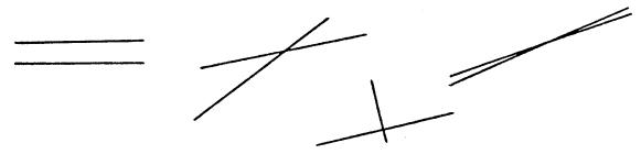
Count as 3 structures if space between fibers is greater than width of 1 fiber diameter or if the number of intersections is equal to or less than 2.
