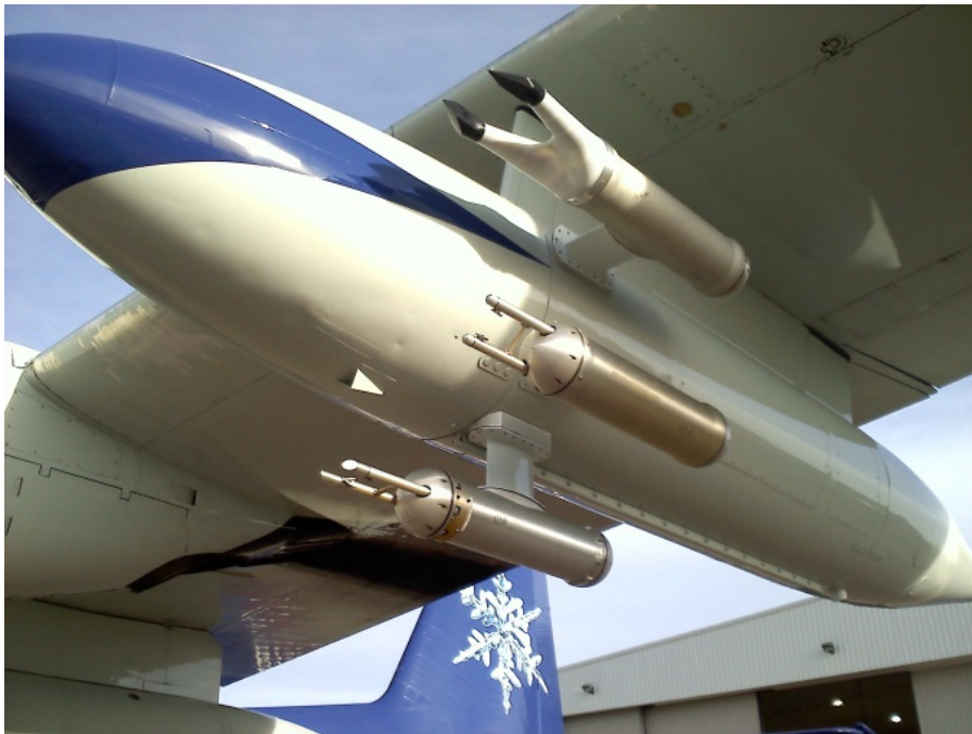
Figure 1. The HOLODEC 2 instrument, far right, shown mounted on the NSF/NCAR C130 aircraft.
