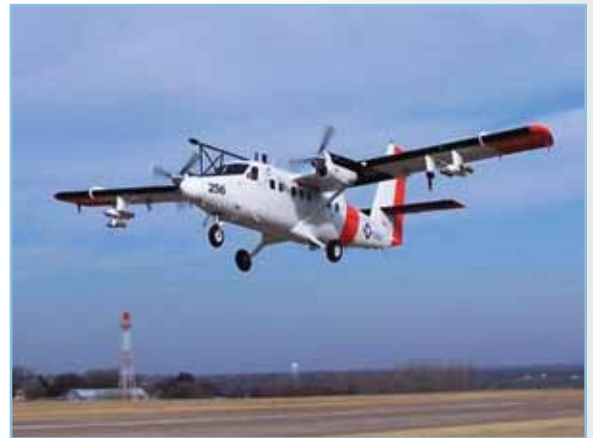
The CIRPAS Twin Otter takes off from Guthrie, Oklahoma, on one of its 59 research flights for RACORO. Cloud and aerosol probes are located under the wings, while radiometers are installed on both the top and bottom of the cabin.
