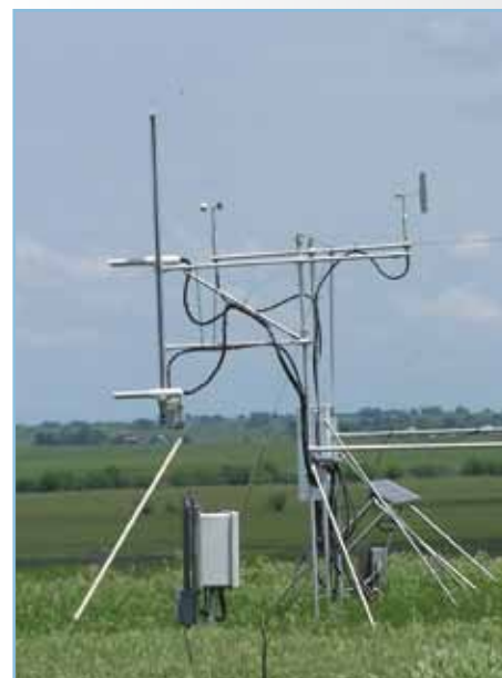
Each EBBR system produces estimates of the vertical fluxes of sensible and latent heat from observations of net radiation, soil surface heat flux, and vertical gradients of temperature and relative humidity.
