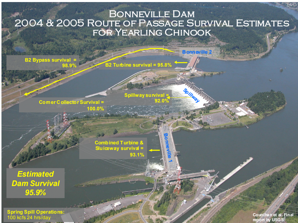
Salmon and steelhead have several ways to pass each dam, including new systems that make passage safer for fish.
