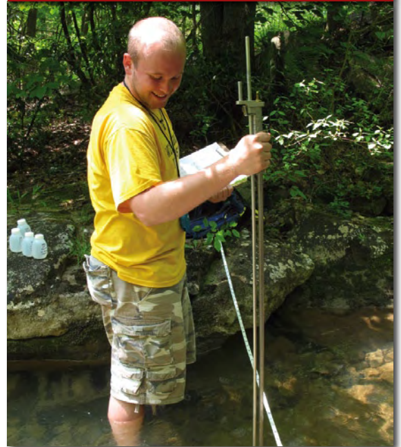
Associate Bryan Olejasz operates a flow meter as part of a water quality monitoring program. Bryan served at a nonprofit watershed group, Friends of Deckers Creek, in Dellslow, WV.
