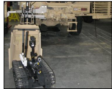
The Robot Deployment System enables Soldiers to deploy and operate road clearance robots safely.
