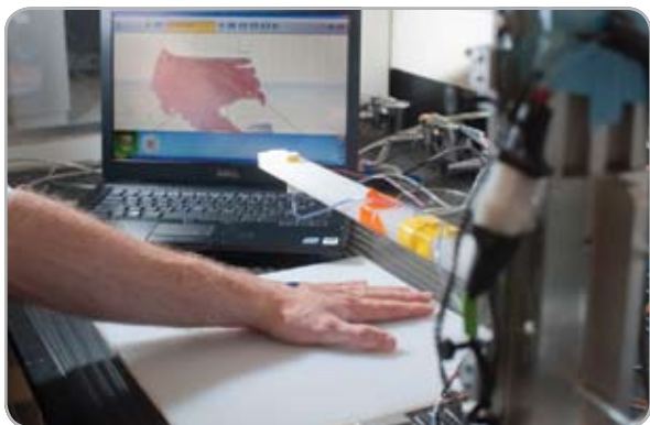
WFPC researchers have developed a prototype system that uses ink jet technology to print skin cells directly on burns.
