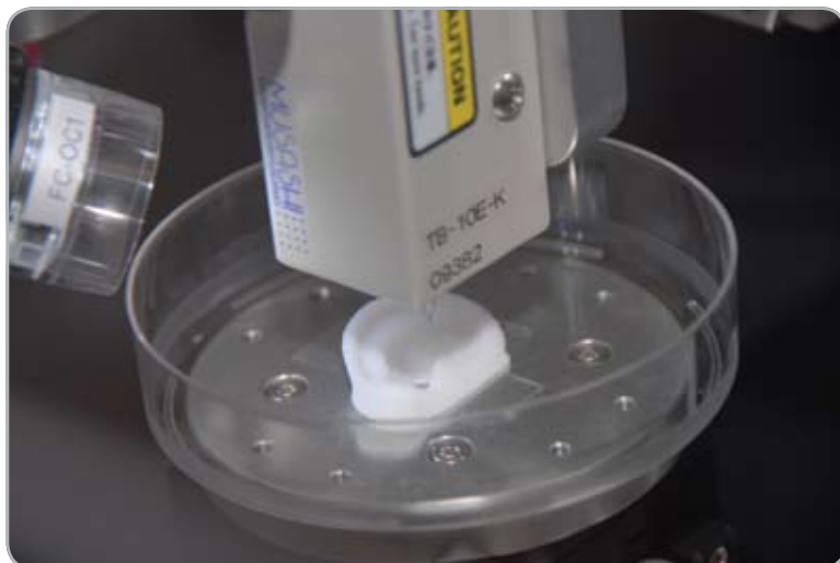
Closeup of a fabricated ear scaffold created by AFIRM researchers.
