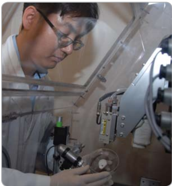
Hung-wok Park fabricating an ear scaffold (WFPC).
