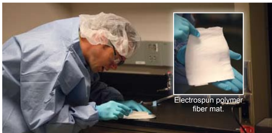
Rutgers University graduate student Charles Florek separates an electrospun polymer fiber mat from a stack of mats that he has prepared for use in animal studies.
