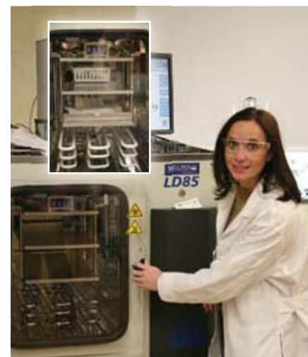
Jenny Raynor, PhD, a postdoctoral associate in Dr. Kohn's laboratory (RCCC), using the lyophilizer to form bone regeneration scaffolds.
