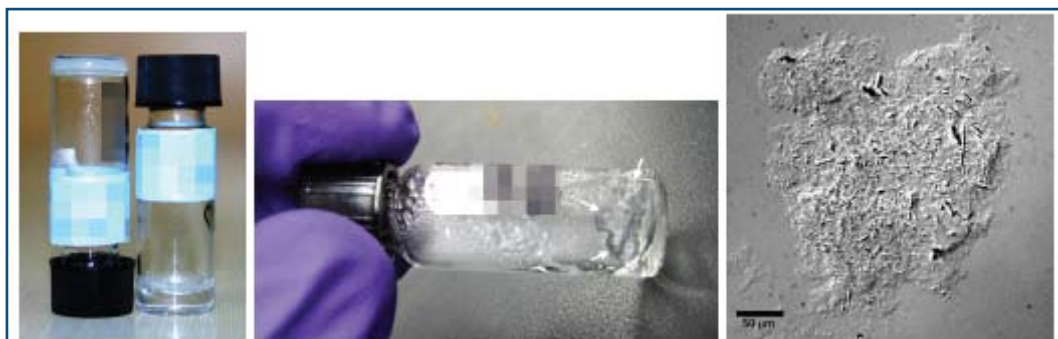
Figure II-28. Gelled PA siC16-W3K. Photograph of PA siC16-W3K gelled (left) after 1 hour incubation at 60°C (20 mg/mL). At lower concentrations, siC16-W3K (1 mg/mL) will remain an aqueous solution with gels (allows) forming slowly over a 24-hour period at 60°C (middle). Microscope image of a siC16-W3K PA gel fixed with glutaraldehyde. Substructures are visible at the micron size range (right).
