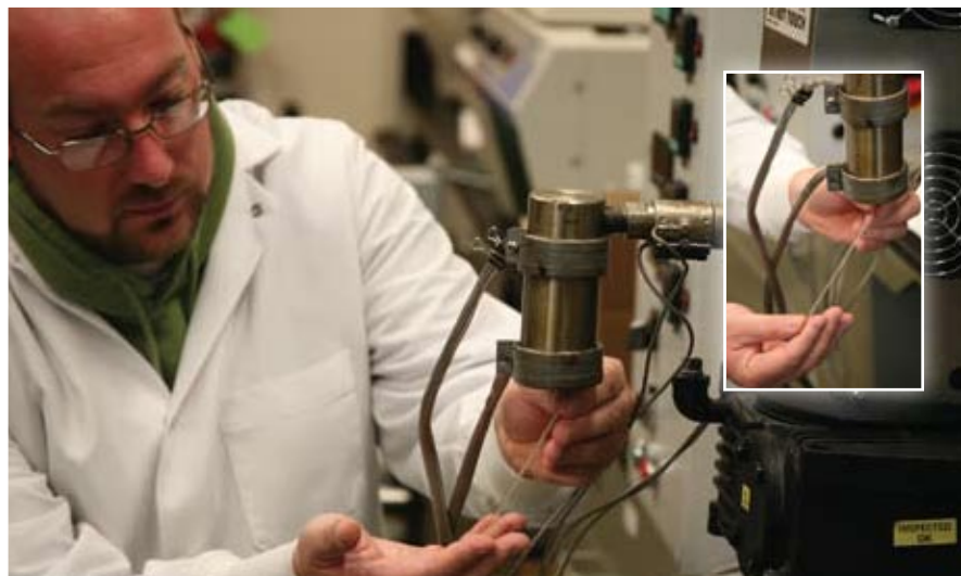
Asa Vaughan, PhD, a postdoctoral fellow in the Kohn laboratory (RCCC), holding an extruded polycarbonate bone pin.
