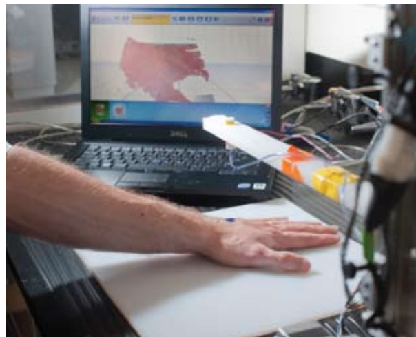
A prototype system has been developed that uses ink-jet technology to print skin cells directly on burns (WFPC).
