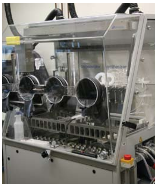
A polymer synthesis robotic accelerator at Rutgers – The State University of New Jersey.
