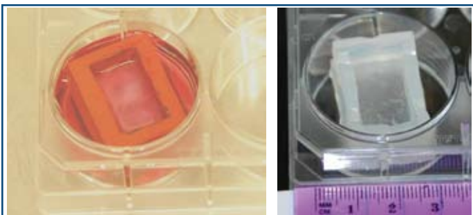
Figure III-16. Picture of the custom-made seeding chamber containing a scaffold in the center of the chamber in a 6-well plate. In this scenario, the seeding chamber is draped with the BAM.
