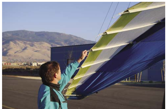
Figure 5-46. Inspecting the trailing edge of the wing.
