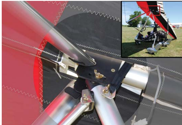
Figure 3-19. Hang point wing attachment.
