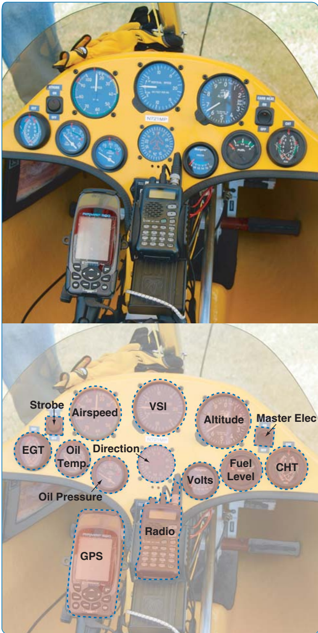
Figure 3-45. Full analog instruments.
