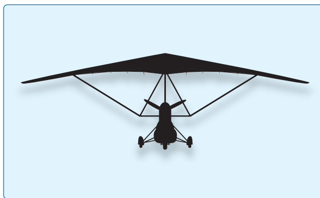
Figure 2-15. Front view with projected area shown that produces drag.
