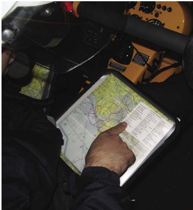
Figure 12-8. Reviewing before-takeoff checklist, which is included for the flight with the sectional charts on the kneeboard.
