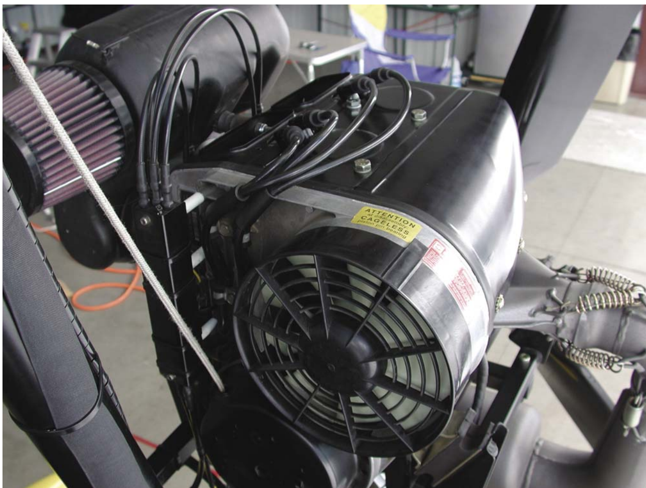
Figure 4-1. Two-stroke air-cooled engine.
