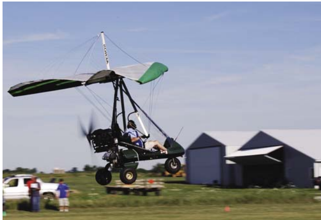
Figure 7-4. Initial takeoff grass strip with control bar pulled in slightly for a higher speed after liftoff in case of engine failure.
