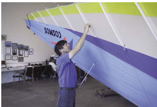
Figure 5-28. Installing the lower surface battens.
