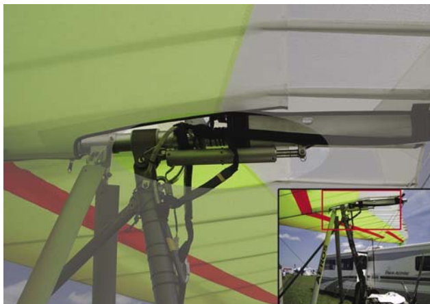
Figure 3-23. Hydraulic inflight trim systems that move the hang point in flight controlled by the pilot.
