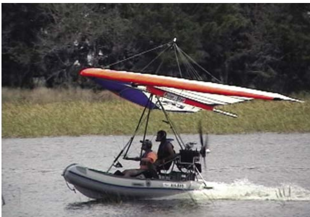
Figure 1-15. WSC aircraft with struts similar to those on an airplane (top) and WSC aircraft operating on water (bottom).
