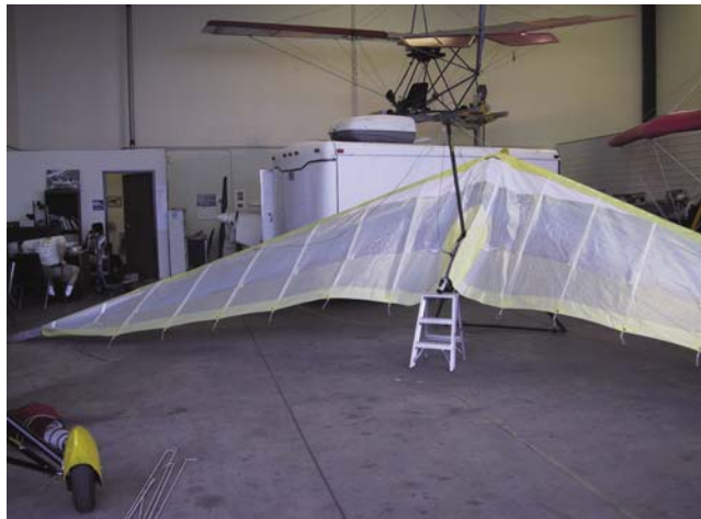
Figure 5-23. Wing ready to tension.
