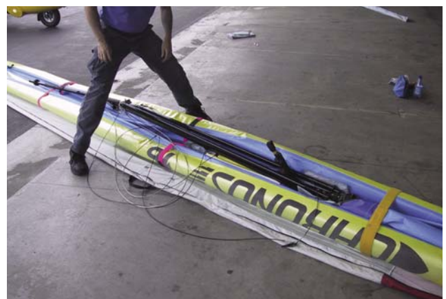
Figure 5-37. Control bar folded down along leading edges but wires not yet organized.
