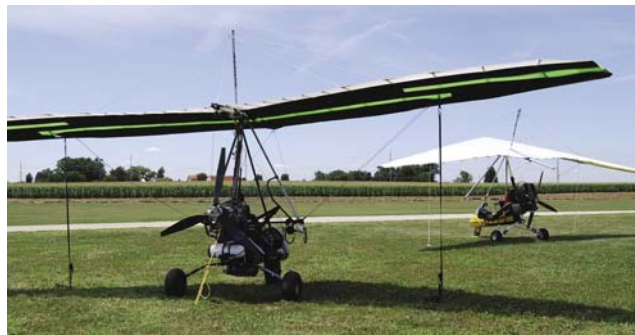
Figure 5-69. Typical tie down for light wind. Left hand WSC control bar pulled back to lower nose for possible headwind, right hand control bar fastened to front tube.
