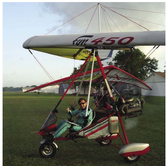
Figure 2-17. Fast WSC aircraft with complete streamlining (top) and slow WSC aircraft with minimum streamlining (bottom).
