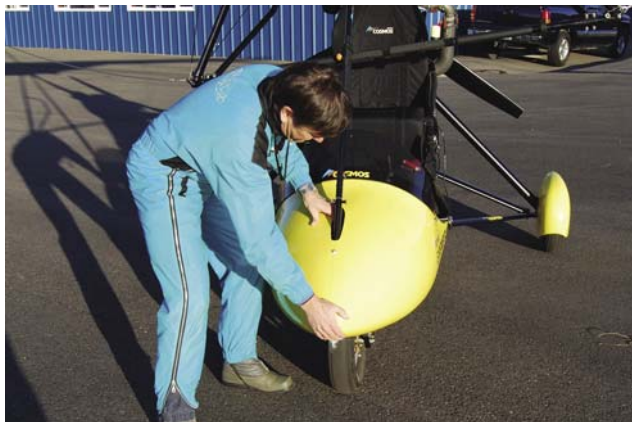
Figure 5-52. Checking the cowl attachment for security and cracks.
