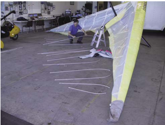
Figure 5-20. Wings spread and battens organized to insert into wings. Note small stepladder holding up keel.
