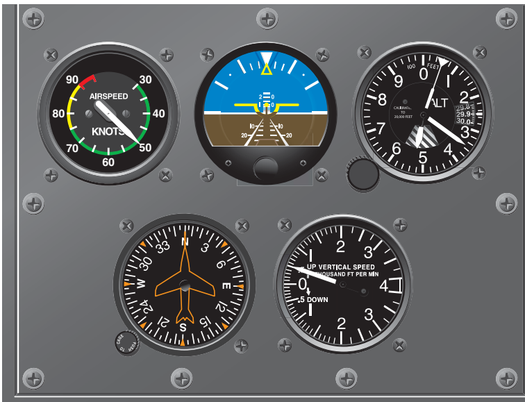
Figure 12-9. Classic instrument gauges for WSC aircraft.
