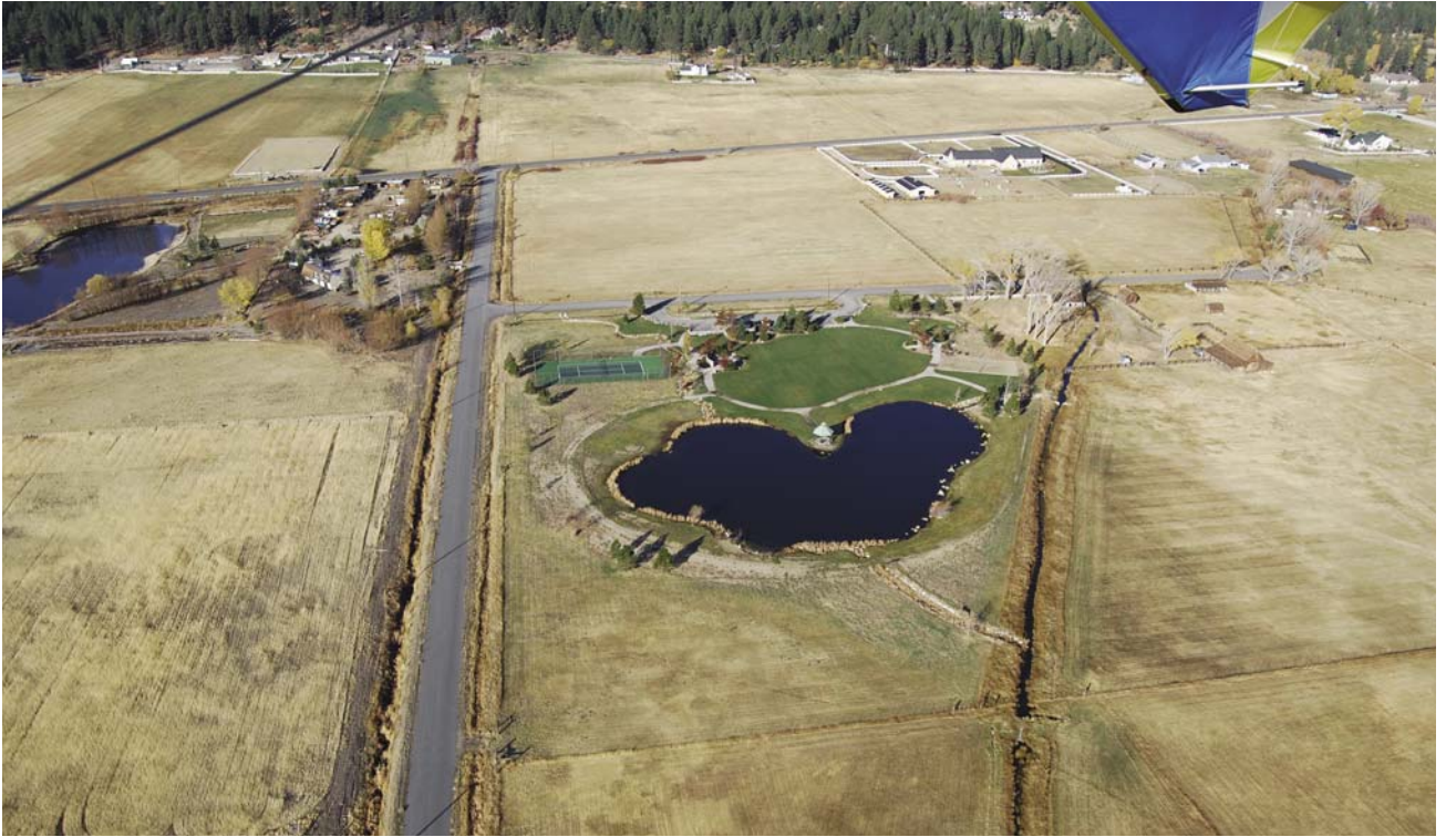
Figure 9-11. Downwind portion of turn about a point, which is the gazebo jutting out into the lake. Notice the wing is low on the downwind portion where the angle of bank is greatest.
