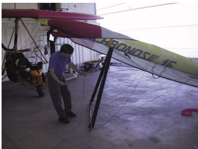
Figure 5-15. Placing the front wires at the control frame.
