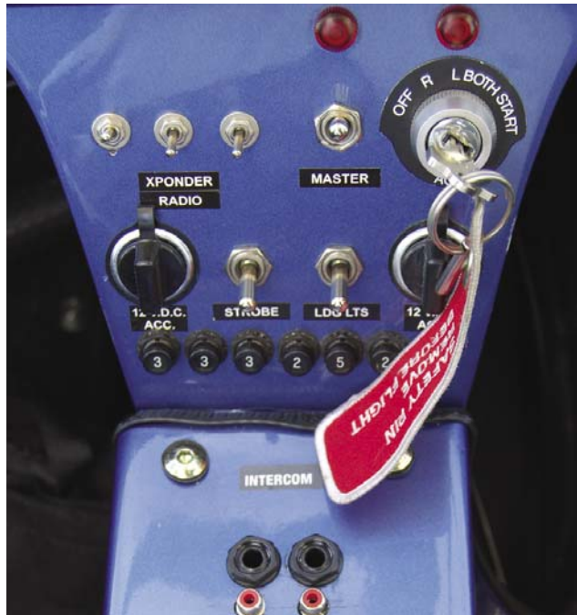
Figure 4-16. Keyed ignition system with integral starter.
