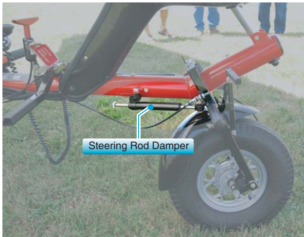
Figure 3-29. Steering rod damper.
