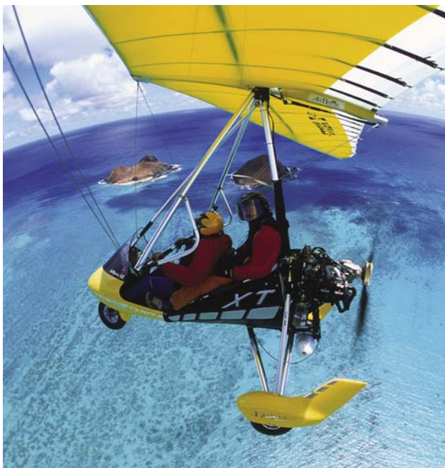
Figure 2-34. Wheel fins for carriage yaw stability.
