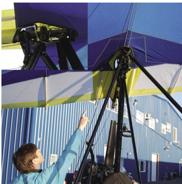
Figure 5-48. Inspecting the wing attachment to the carriage.
