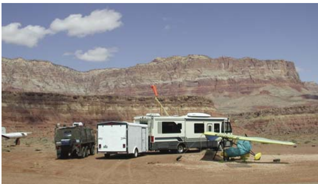
Figure 5-73. Wing lowered and four point tie-down with carriage cover to protect flight deck and engine.
