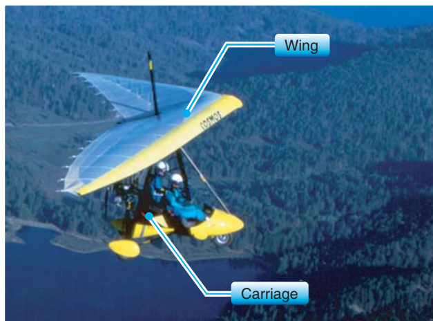
Figure 1-13. Carriage and wing of a WSC aircraft.
