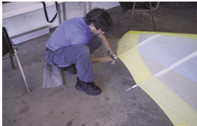
Figure 5-27. Installing the wing tip battens.
