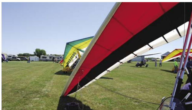
Figure 5-71. Wing tied down with tip on ground into wind.
