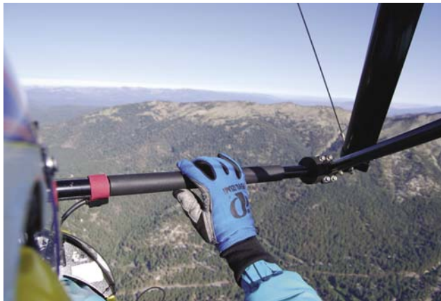
Figure 6-3. Hold the control bar with a light touch to feel every movement in the wing.
