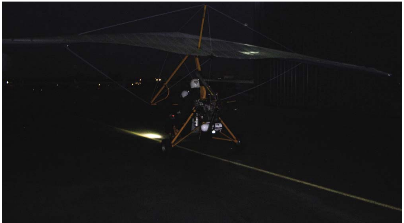
Figure 12-4. Landing light on WSC aircraft taxiing at night.
