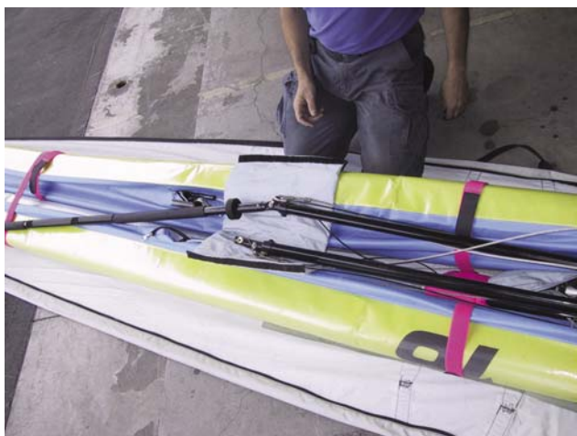
Figure 5-12. Wing cover bag unzipped, showing unique padding around control frame corner brackets.
