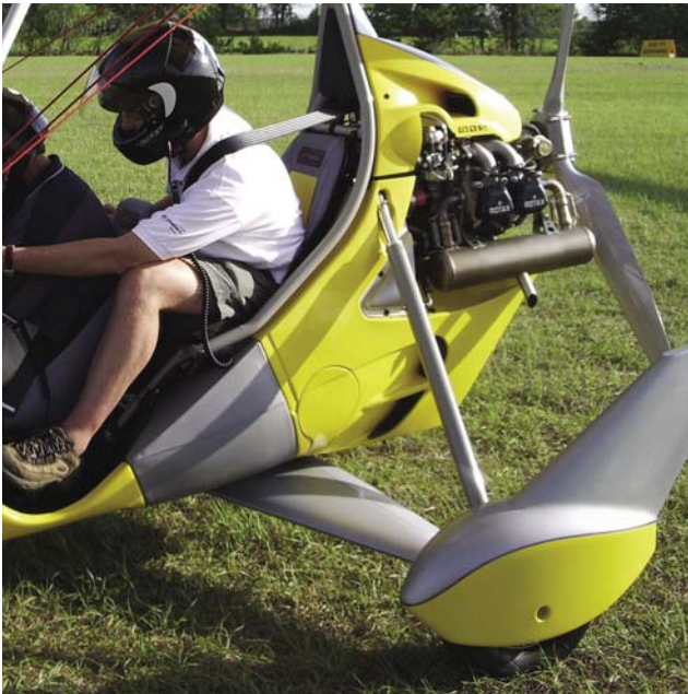
Figure 3-36. Conventional landing gear with streamlined drag and main struts.
