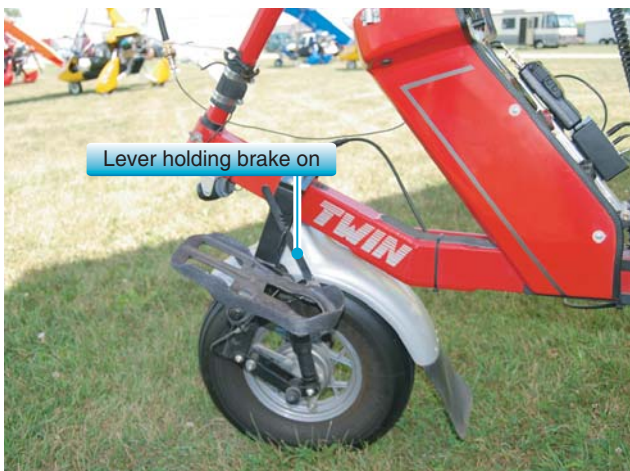
Figure 3-32. Mechanical parking brake system.
