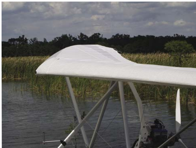
Figure 3-10. Clean upper surface of strutted wing.
