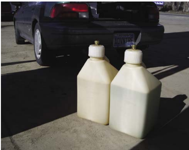
Figure 4-19. With these translucent containers, it can be noted that the left hand container is just auto fuel and the right hand container shows the auto fuel is premixed with oil for a two-stroke engine.
