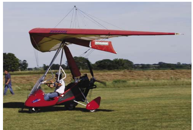
Figure 2-33. Keel pockets and vertical stabilizers are additional tools designers use for yaw stability on the wing.
