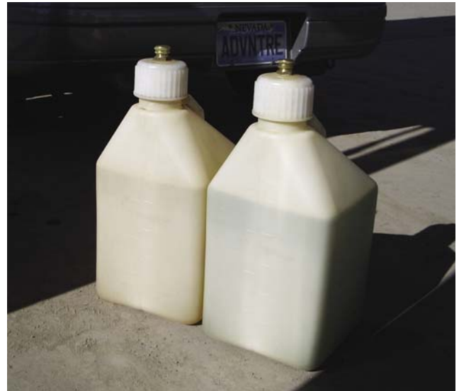
Figure 5-59. Translucent fuel containers with premixed oil (right) and auto gas only (left).
