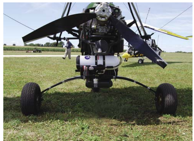
Figure 3-35. Solid flexible main gear.
