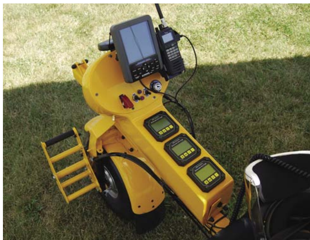
Figure 3-27. Large foot rests used for steering the aircraft on the ground (left hand ground brake shown).
