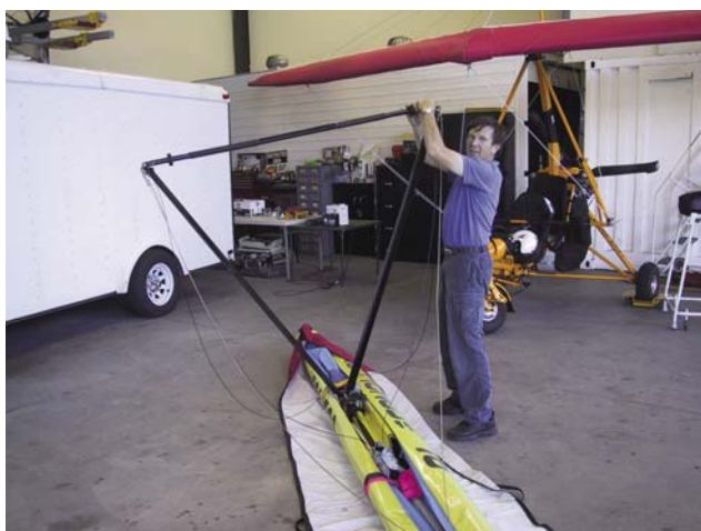
Figure 5-13. Assembling control frame.
