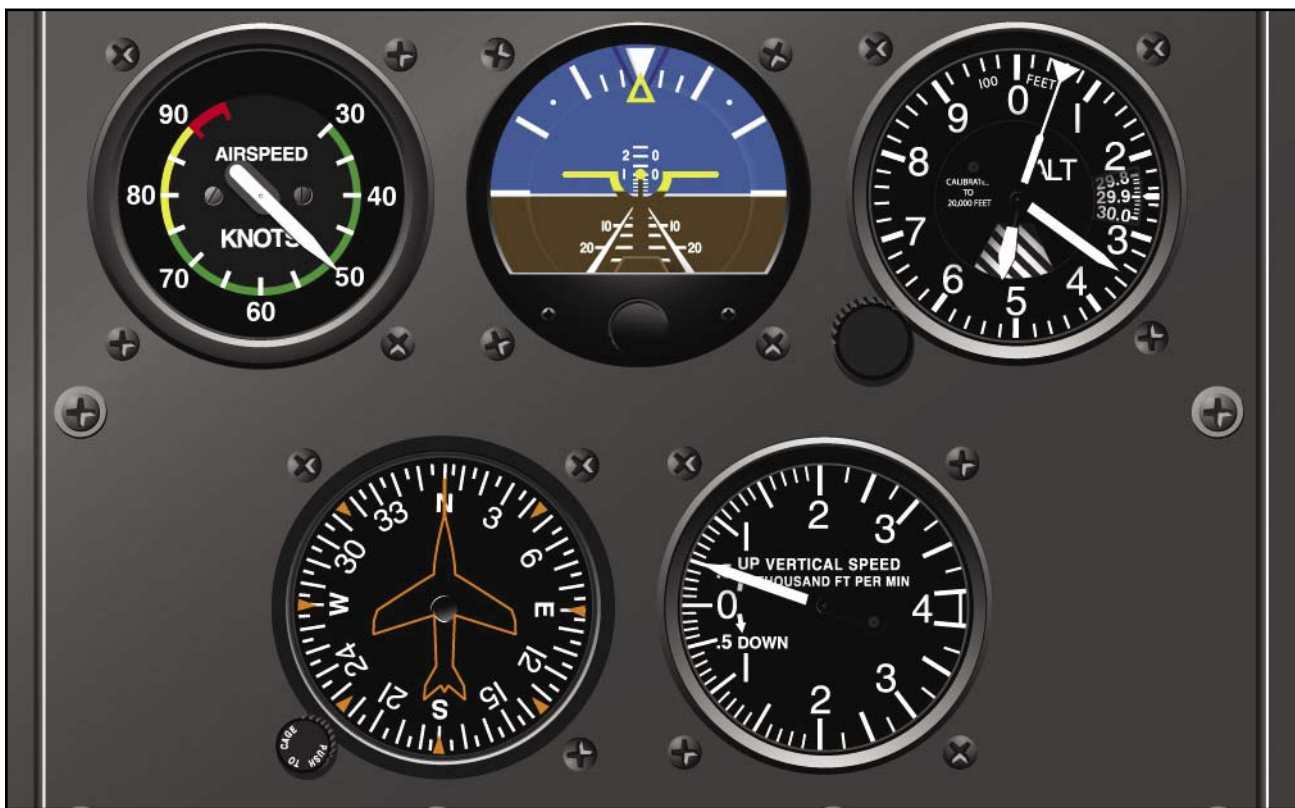
Figure 13-9. Optional analog gauges for instrument flying; attitude indicator (top middle) and direction indicator (lower left) not typically installed on WSC aircraft.
