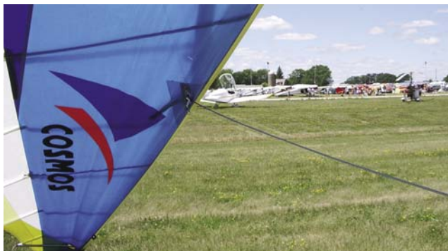
Figure 5-70. Pilot's view of the left hand wing lowered into the wind, allowing the pilot to exit the aircraft in higher winds with the wind pushing down on the wing from the side.
