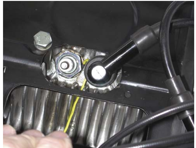
Figure 4-20. Cylinder head temperature probe (yellow wire) is under spark plug.
