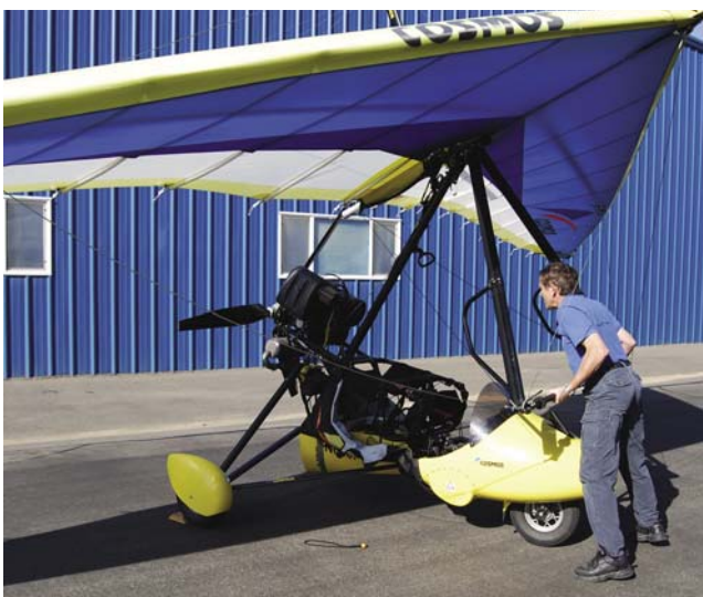
Figure 5-31. Lifting the wing up into position.
