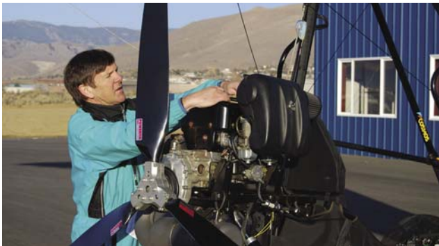
Figure 5-56. Checking spark plug cap security to the spark plugs.
