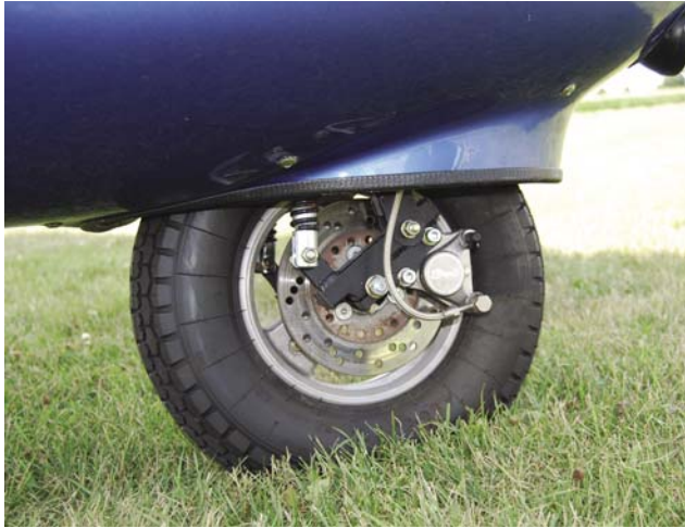
Figure 3-31. Hydraulic disk brake system.
