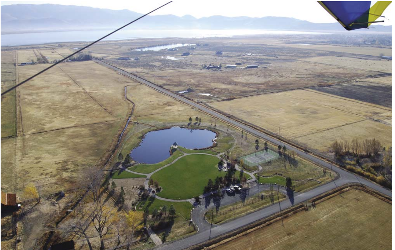
Figure 9-12. Upwind portion of the turn about a point. Notice the wing is higher because bank angle is not at as steep during the upwind portion headed into the wind to maintain a constant radius circle.
