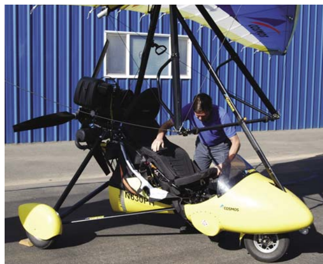
Figure 5-33. Installing the seats.
