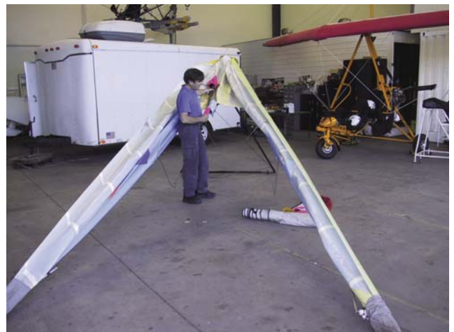
Figure 5-17. Wings spread slightly to raise the kingpost.
