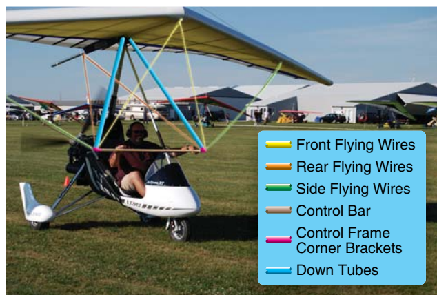
Figure 3-6. Control frame with downtubes, control bar, and corner bracket with flying wing wires, and control frame fore and aft wires.
