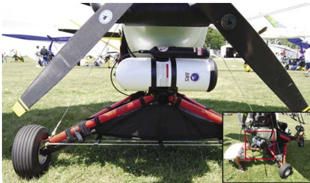
Figure 3-42. Canister mounted under engine.
