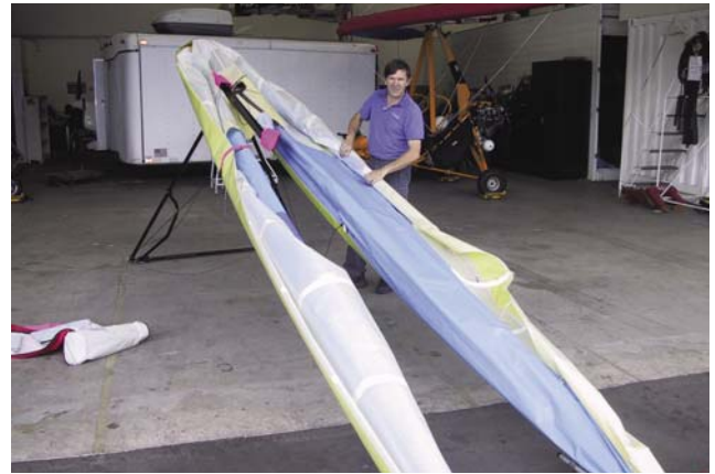
Figure 5-35. Left hand side rolled up and secured with wing tie. Rolling right hand sail which will also be secured with wing tie.
