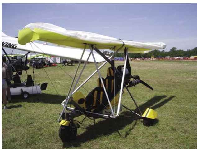
Figure 3-9. A strutted wing folded back so it can fit into a trailer for storage and easy transport (top). Strutted wing with wings folded back for easy storage (bottom).
