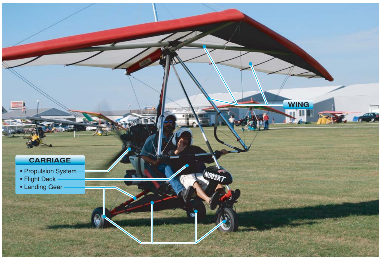
Figure 3-1. Wing and carriage of WSC aircraft.
