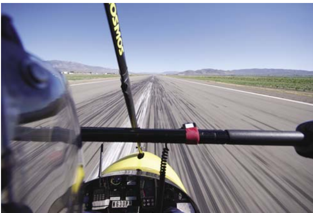
Figure 11-14. Completing the roundout with the control bar full forward and the back wheels settling to the runway.
