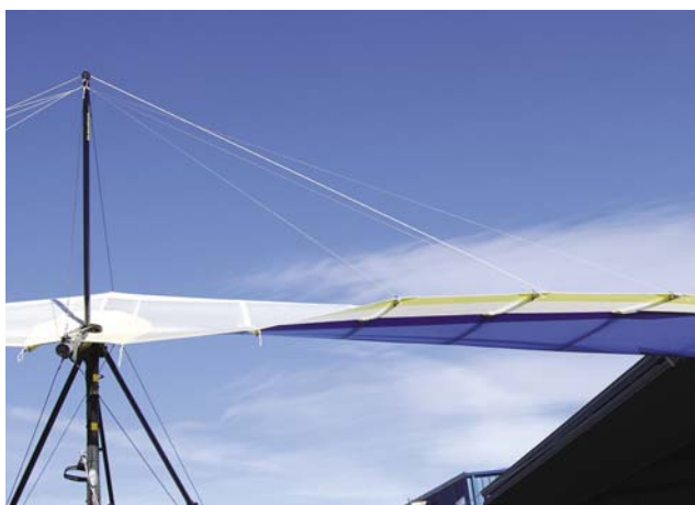
Figure 5-47. Inspecting the kingpost, top wires, and crossbar tension hardware.
