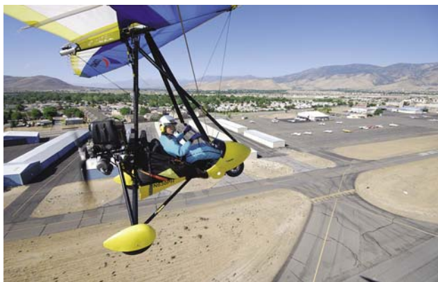
Figure 7-5. Best climb speed control bar position for this WSC is shown after initial climb where there is sufficient altitude for easy recovery in case of engine failure.
