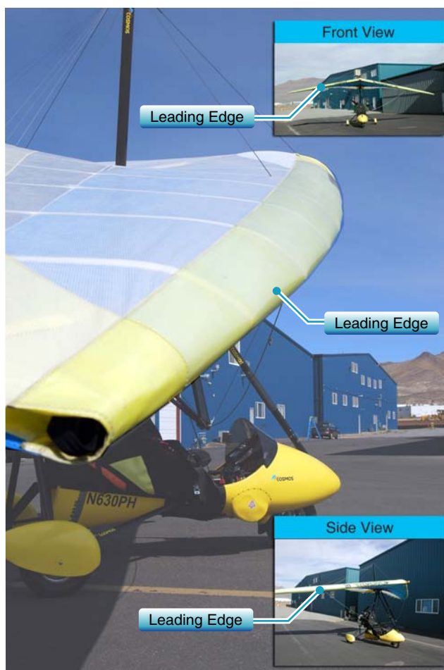
Figure 3-11. Curved leading edge sail design.
