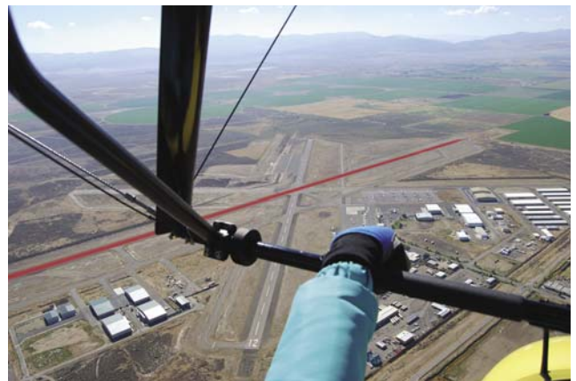
Figure 10-9. After hearing other aircraft using the normal pattern as described in the Airport/Facility Directory (A/FD), pilot descended and entered the downwind leg (landing runway highlighted in red) midfield within gliding distance of the runway in case of an engine failure.
