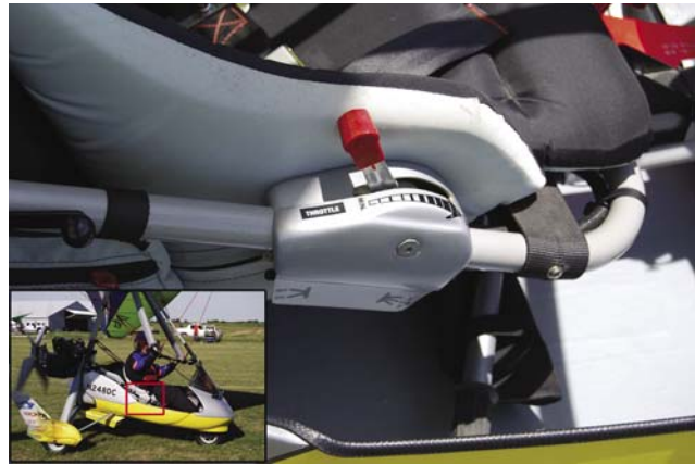
Figure 3-43. Cruise throttle control and ignition switches.
