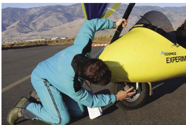
Figure 5-50. Checking the front wheel, tire, and front fork assembly.
