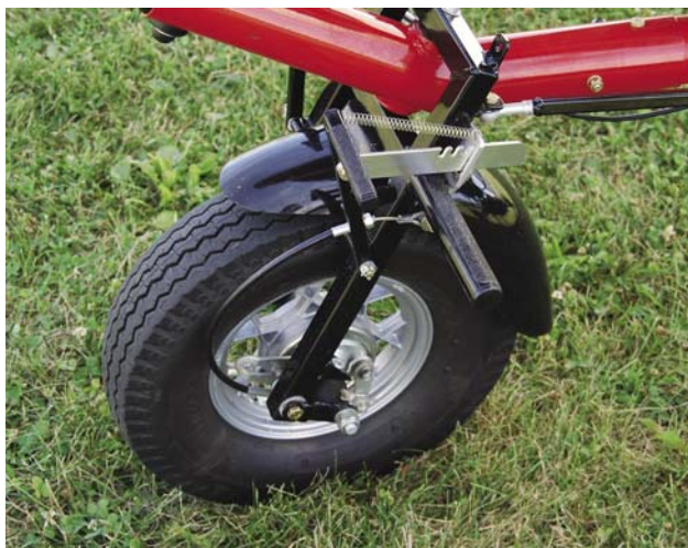
Figure 3-30. Mechanical drum brake system.
