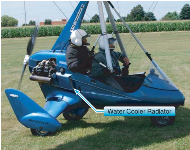
Figure 4-22. Side mounted water cooler radiators integral with cowl.
