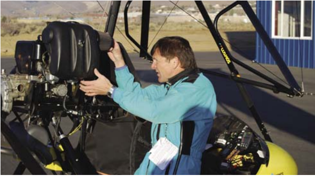
Figure 5-55. Checking the security of the air inlet filter and the security of the carburetors to the engine.
