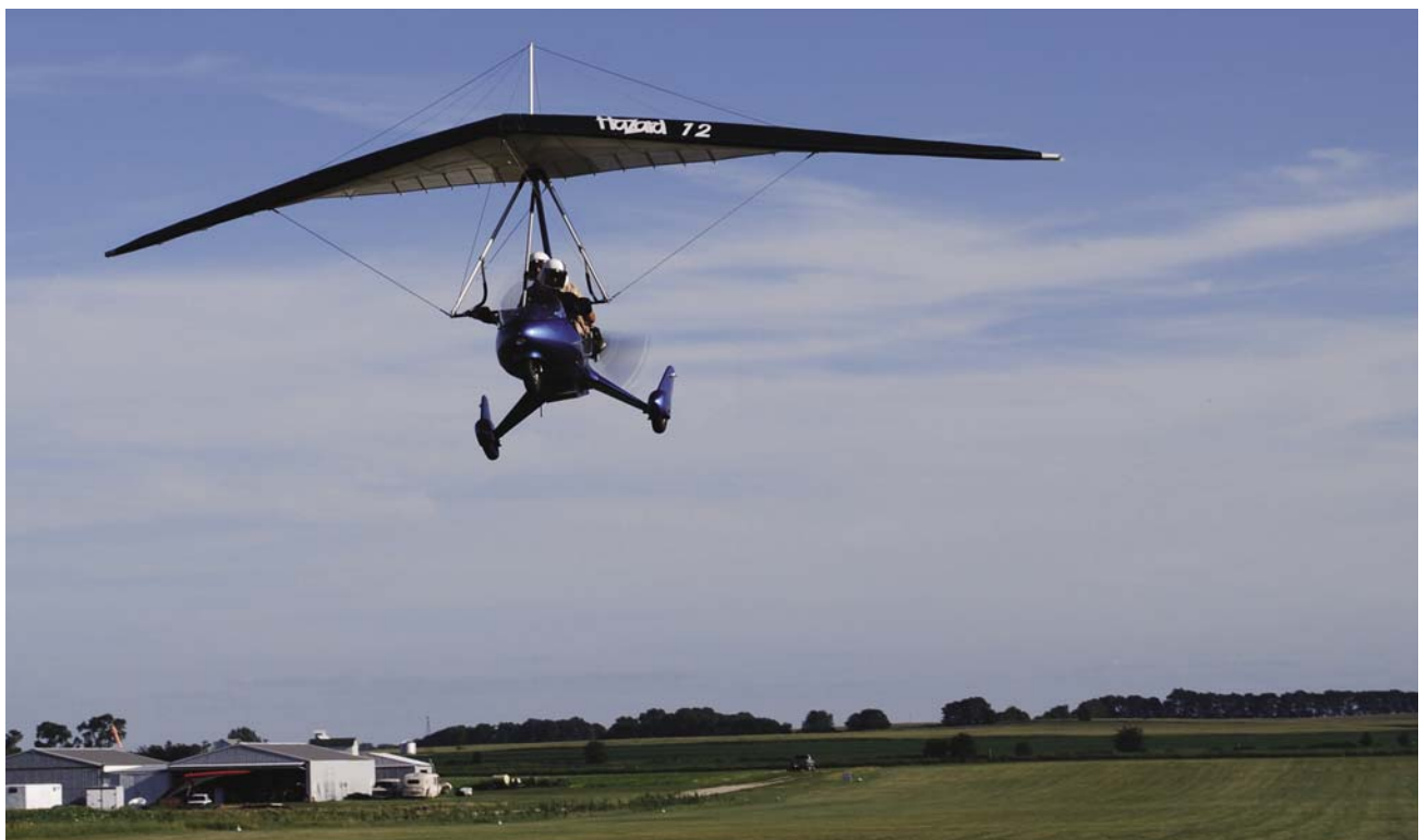
Figure 7-13. Grass fields are commonly used for WSC operations but require a longer time to accelerate to takeoff speed.
