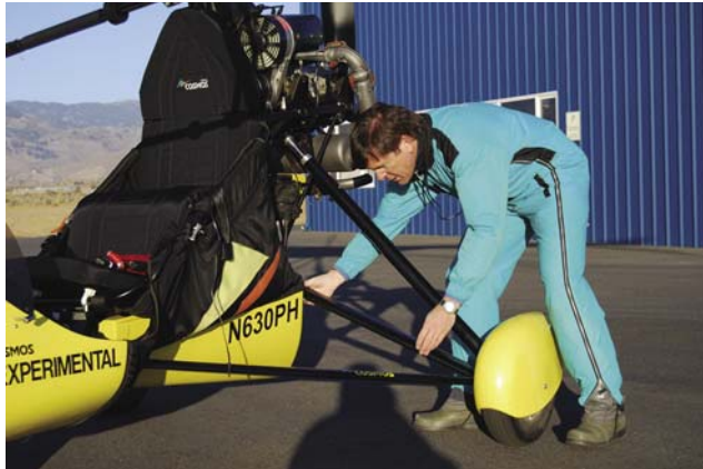
Figure 5-51. Checking the rear landing gear struts.
