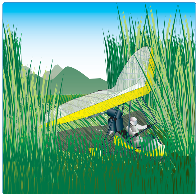
Figure 13-2. Using vegetation to absorb energy.
