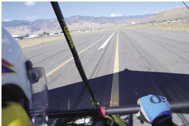
Figure 5-68. After landing, the pilot slows to the appropriate taxi speed before following the yellow taxi lines to exit the runway.
