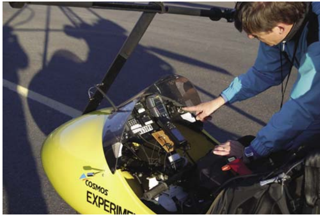
Figure 5-58. Checking the flight deck instruments for readability and security. Turning on the main electrical power to verify proper instrument readings.
