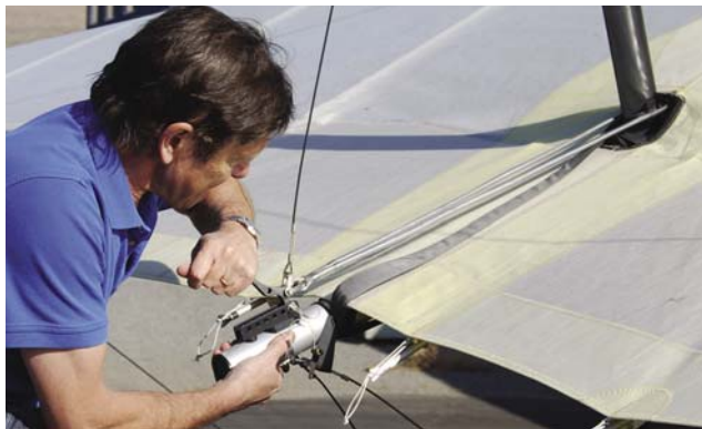
Figure 5-24. Attaching the tensioning cables to the back of the wing to complete the wing tensioning step.
