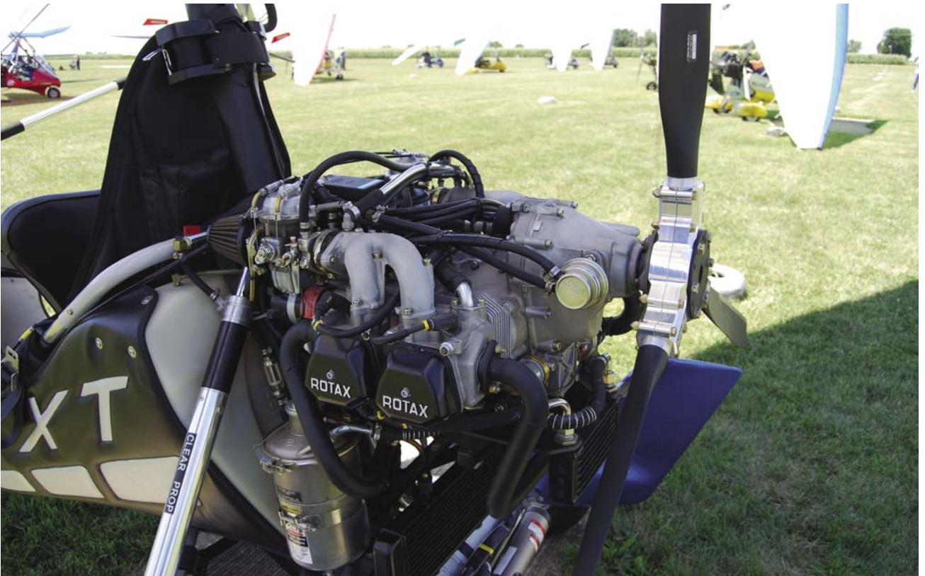
Figure 4-3. Four-stroke water- and oil-cooled engine.
