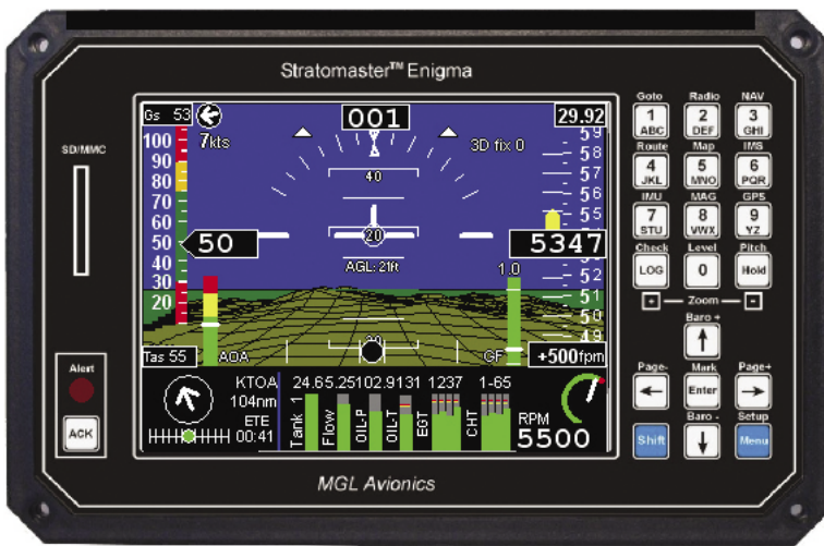
Figure 12-10. Digital panel instrument gauges for WSC aircraft.
