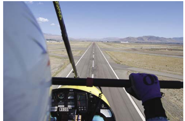
Figure 7-6. Pilots view showing WSC centered in the middle of the runway during initial climb.
