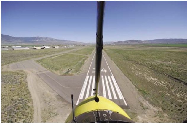
Figure 11-6. Coming to the runway and increasing speed slightly within 50 feet of the ground.
