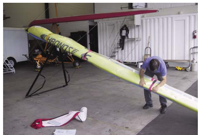
Figure 5-36. Securing both leading edges together so the wing easily fits into the bag.
