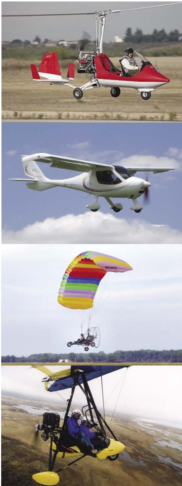
Figure 1-12. Examples of LSA, from top to bottom: gyroplane, airplane, powered parachute, and weight-shift control aircraft.
