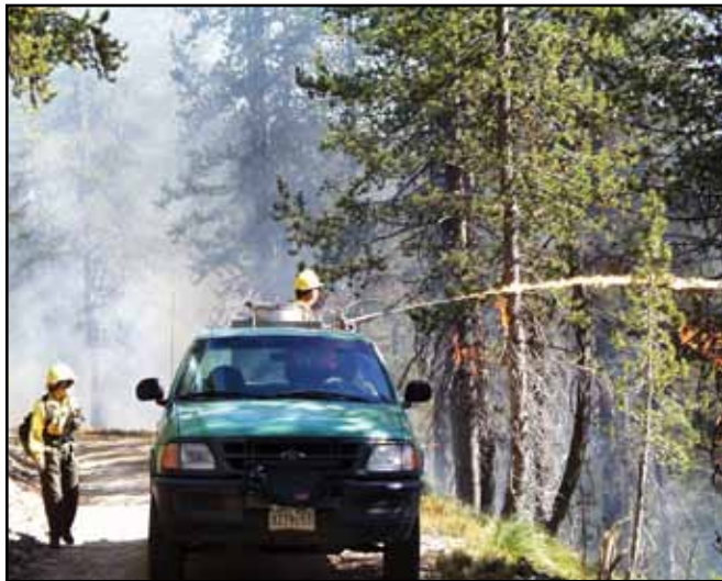
Figure 5. Terra-torch used to ignite the high intensity, stand-replacement prescribed fire at the Beaver Ridge study site.
