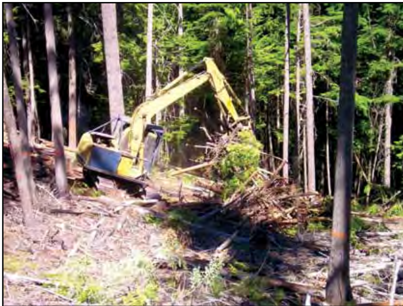
Figure 16. Grapple machines have the ability to separate coarse from fine fuels more readily than tractors and tend to displace and compact soils less than tractors.
