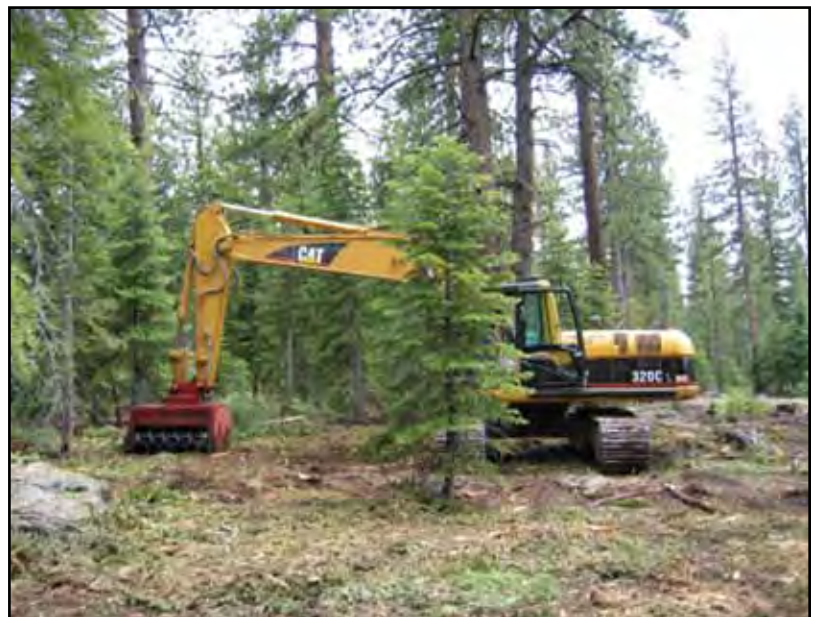
Figure 17. Masticator used to treat ladder and surface fuels in the moist forests near Lake Tahoe, California.
