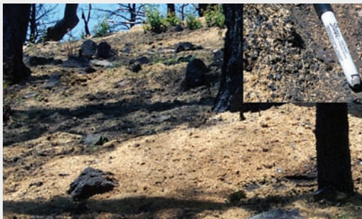
SB3-fig. 3. Pellets of pulverized rice straw and granular PAM were applied dry and compressed and are shown here after a rain expanded the pellets. The insert in the upper right corner shows the small rice straw fibers more closely (felt tip pen inserted for scale).
