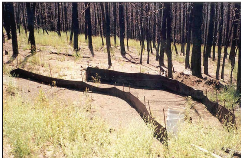
Figure 6. Hillslope plot that incorporates a swale with a double silt fence at the base for sediment collection on the 2000 Bobcat Fire in Colorado.
