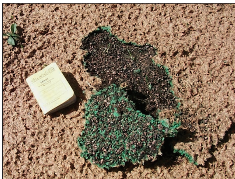
Figure 24. A small piece of the aerielly-applied hydromulch mat (exposed surface is brown) has been lifted off the burned soil (black) and flipped over to expose the underside of the mat (black and green). The pocket-sized field notebook is included for scale.
