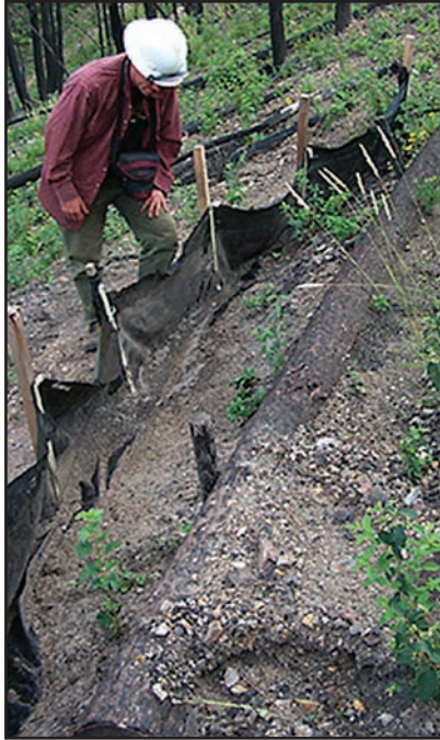
Figure 5. Hillslope plot with a contour-felled log and a silt fence at the base for sediment collection on the 2000 Valley Complex Fires in Montana.
