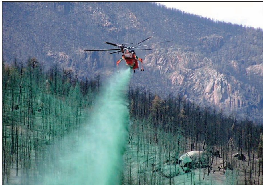
Figure 23. Large-capacity helicopters fitted with slurry tanks are used to apply hydromulch as a post-fire hillslope treatment on the 2002 Hayman Fire in Colorado.
