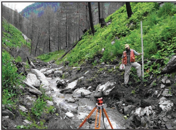
SB1-figure 1. Cross-section measurements were used to model the storm flow and estimate the parameters of the post-fire debris flow in this channel.
