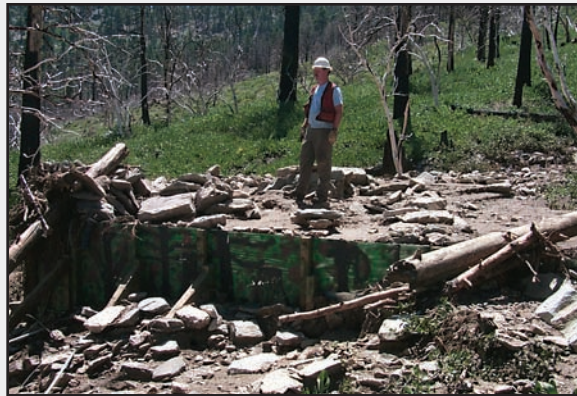
SB5-fig. 1. In post-fire year four, a paired watershed study site on the 2002 Cannon Fire in California had a rainfall event with maximum 10-min intensity ( I_{10} ) of 6.22 \text{ inch h}^{-1} ( 158 \text{ mm h}^{-1} ). The sediment basin filled and then over-topped, depositing large rocks and tree debris both inside and outside the sheet metal wall that forms the sediment basin. The sediment yield from the contour-felled log treated catchment was estimated at over 3.9 \text{ ton ac}^{-1} ( 8.7 \text{ Mg ha}^{-1} ) (see table AB-9 in Appendix B).
