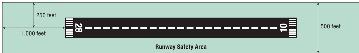
Figure 21 Runway Safety Area
