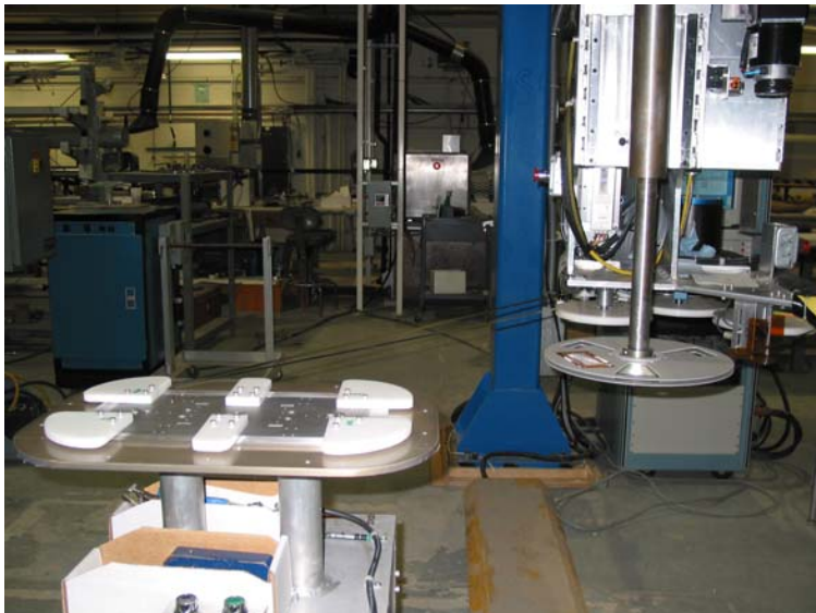
HTS coil winding with SS tape insulator
