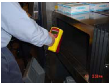
Photos 7-10: NIOSH researchers measuring radiation levels from TRX and EDS machines:
