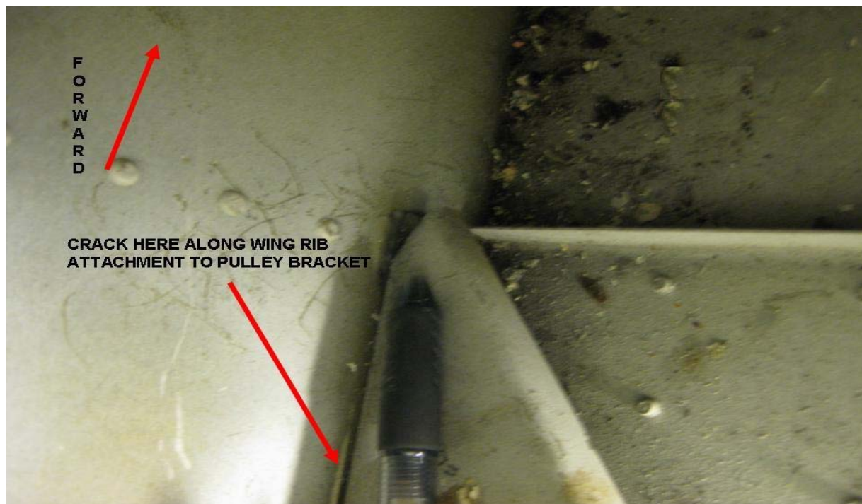
“VIEW LOOKING DOWN ON RIGHT HAND WING FORWARD CORNER OF LOWER PULLEY BRACKET” NOTE*- THE CRACK WAS MORE EVIDENT WITH UPWARD PRESSURE ADDED TO THE TRAILING EDGE OF THE AIRLERON.
