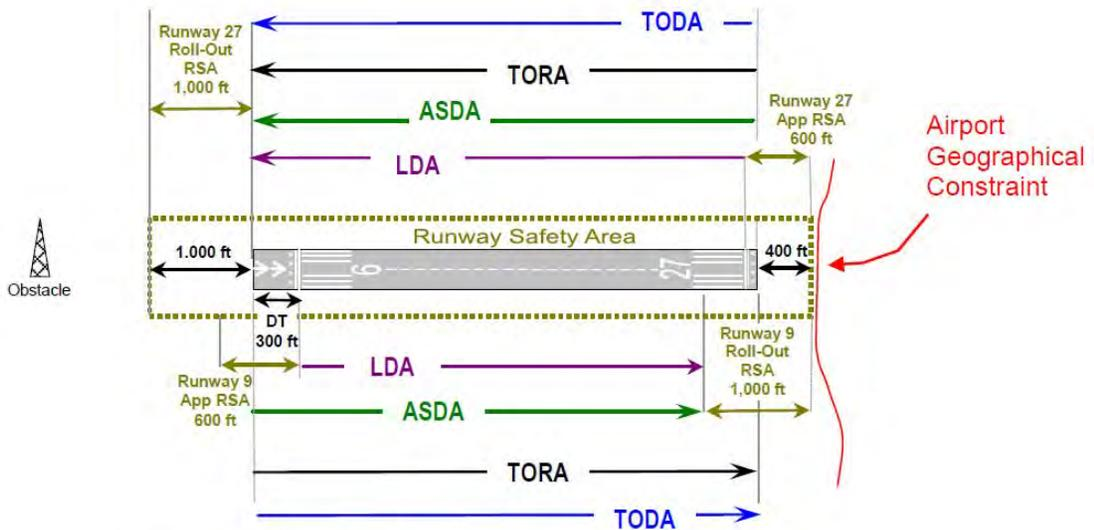
**Runway 9 operations:** The ASDA is reduced by 600 ft to achieve the required RSA at the roll-out end of the runway. The LDA is reduced by 900 ft because, 1) the 300 ft displaced threshold located at the approach end of the runway (due to an approach obstacle), and 2) as result of the 600 ft of runway needed to achieve the required RSA at the roll-out end of the runway.
