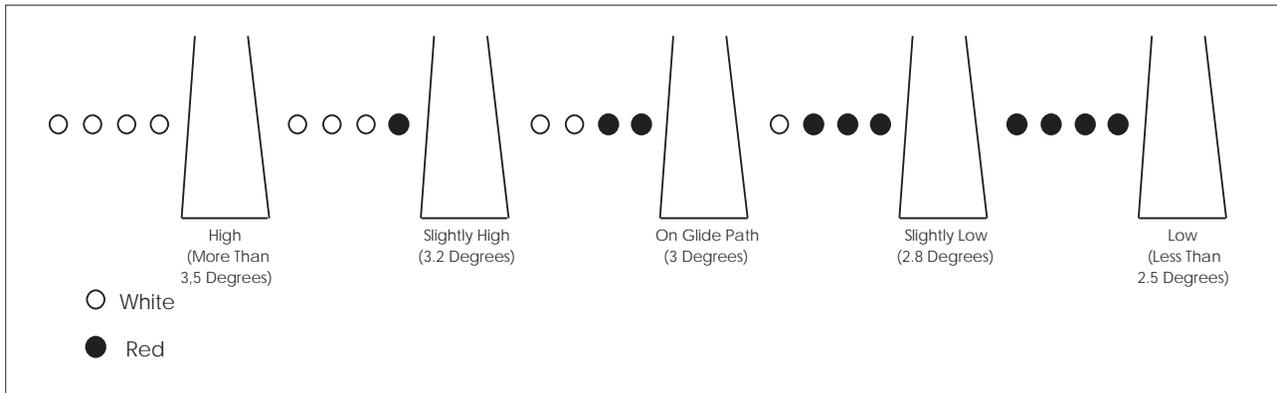
**c. Tri-color Systems.** Tri-color visual approach slope indicators normally consist of a single light unit projecting a three-color visual approach path into the final approach area of the runway upon which the indicator is installed. The below glide path indication is red, the above glide path indication is amber, and
