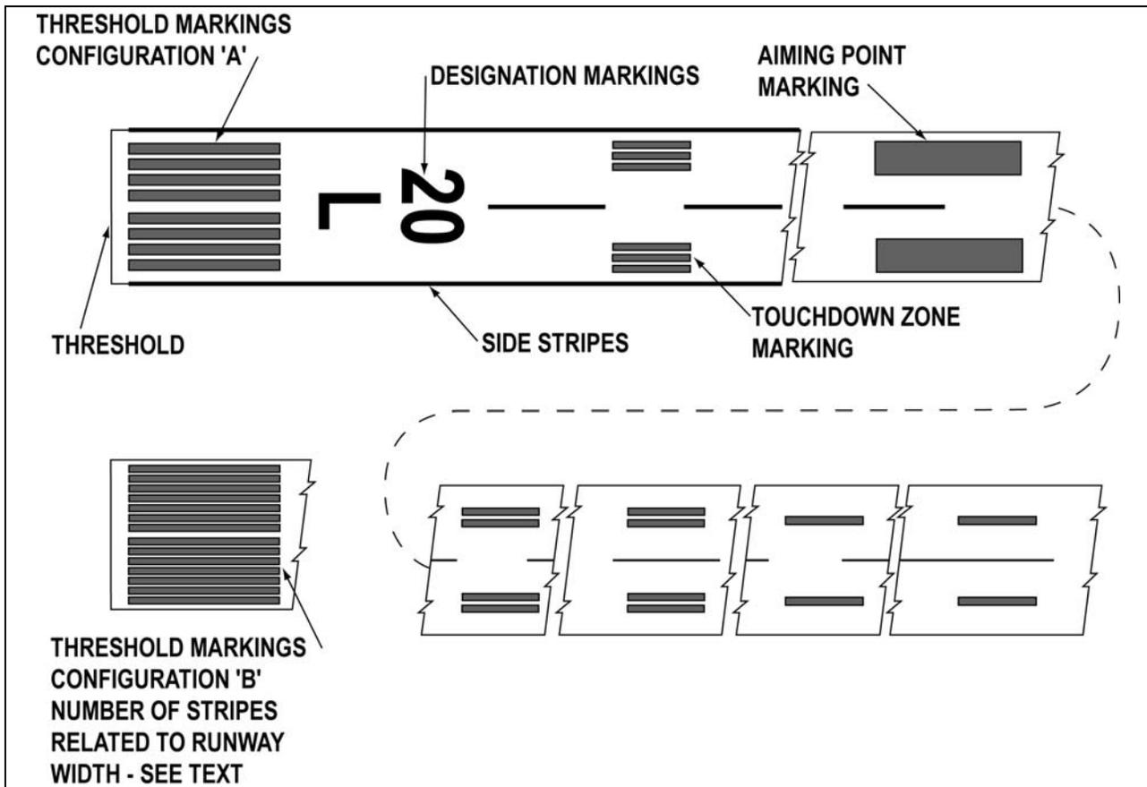
**b. Runway Designators.** Runway numbers and letters are determined from the approach direction. The runway number is the whole number nearest one-tenth the magnetic azimuth of the centerline of the runway, measured clockwise from the magnetic north. The letters, differentiate between left (L), right (R), or center (C), parallel runways, as applicable:
