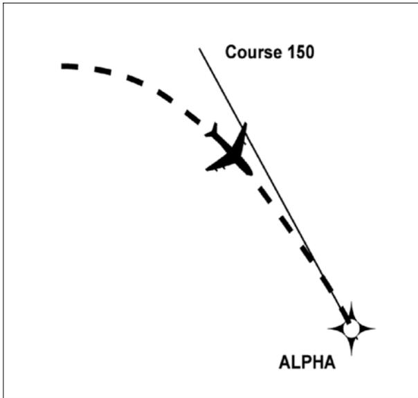
(d) **Radius to Fix.** A Radius to Fix (RF) leg is defined as a constant radius circular path around a defined turn center that terminates at a fix. See FIG 1–2–5.
