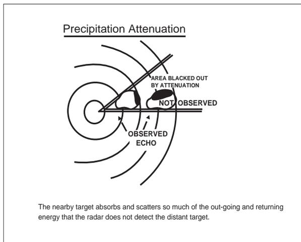
(a) The characteristics of radio waves are such that they normally travel in a continuous straight line unless they are:
