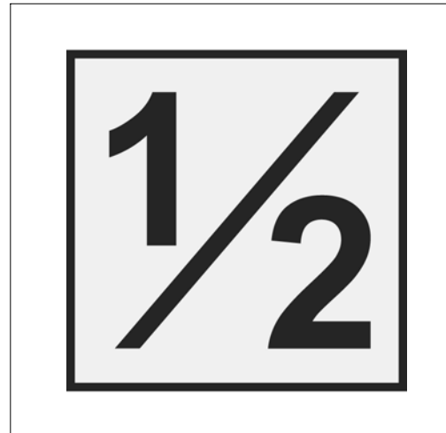
FIG ENR 5.7-1 Typical Runway Half-way Sign
