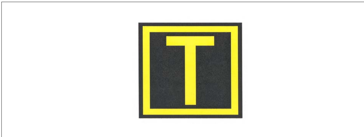
FIG AD 1.1-42 Taxiway Location Sign
