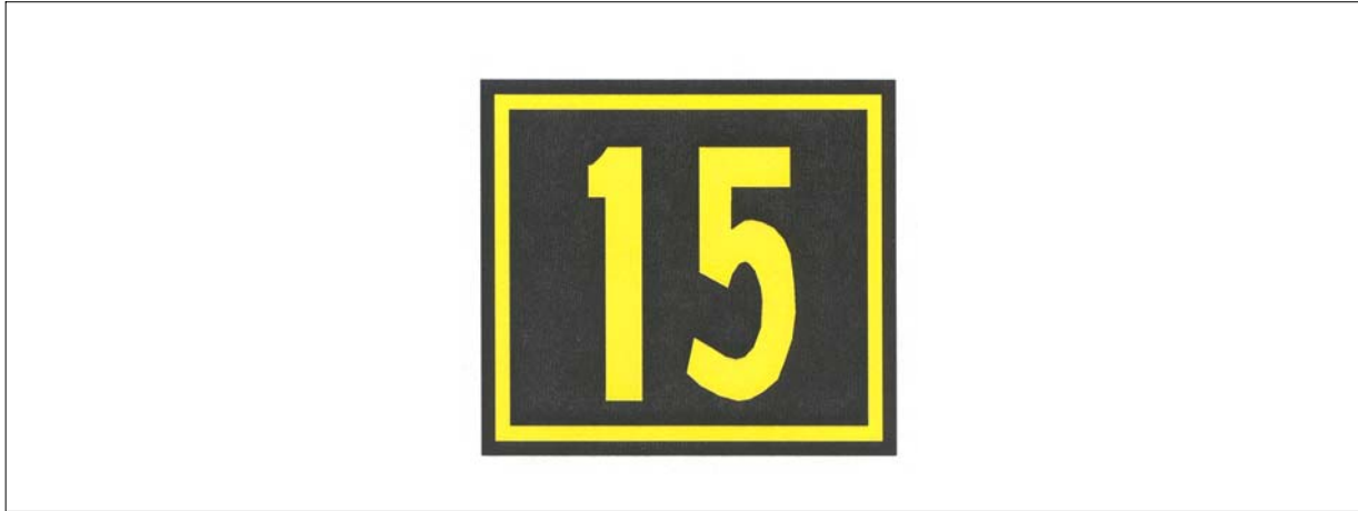
FIG AD 1.1-44 Runway Location Sign
