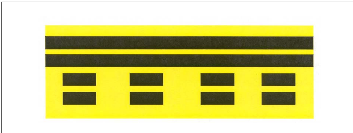
FIG AD 1.1-45 Runway Boundary Sign
