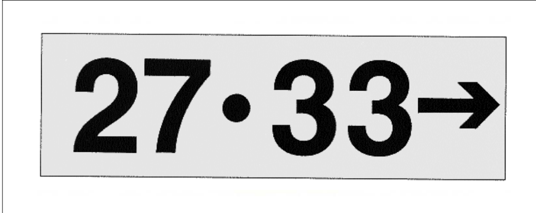
FIG AD 1.1-51 Destination Sign for Common Taxiing Route to Two Runways
