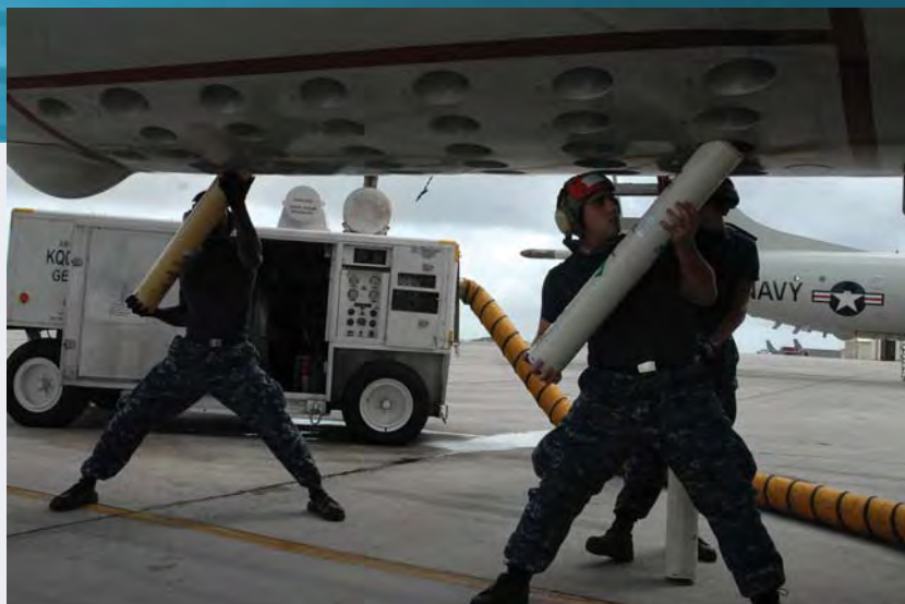
Sailors load sonobuoys before flight operations on a P-3C Orion. DLA Troop Support's Clothing and Textile Division is developing a bio-degradable parachute for sonobuoys, which are a sonar canister system ejected from air craft or ships that deploy as a buoy upon water impact. Photo by Navy Petty Officer 2nd Class Julian R. Moorefield
