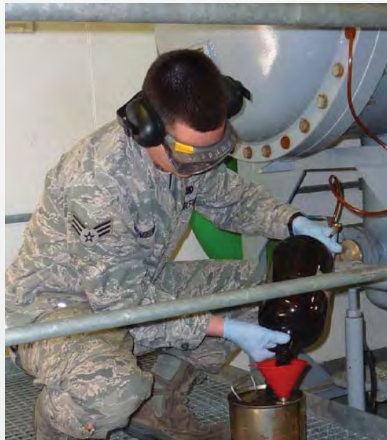
An Airman collects fuel for testing at the fuels control center of the 86th Logistics Readiness Squadron/ Logistics Group Readiness Flight at Ramstein Air Base, Germany.
