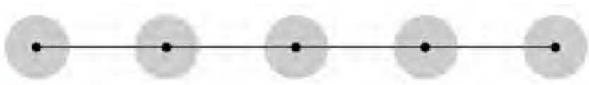
Figure H-3. Schematic of a point-transect depicting a cluster of five, 1/5th acre plots spaced four chains (264 ft) apart upon which habitat metrics were sampled
