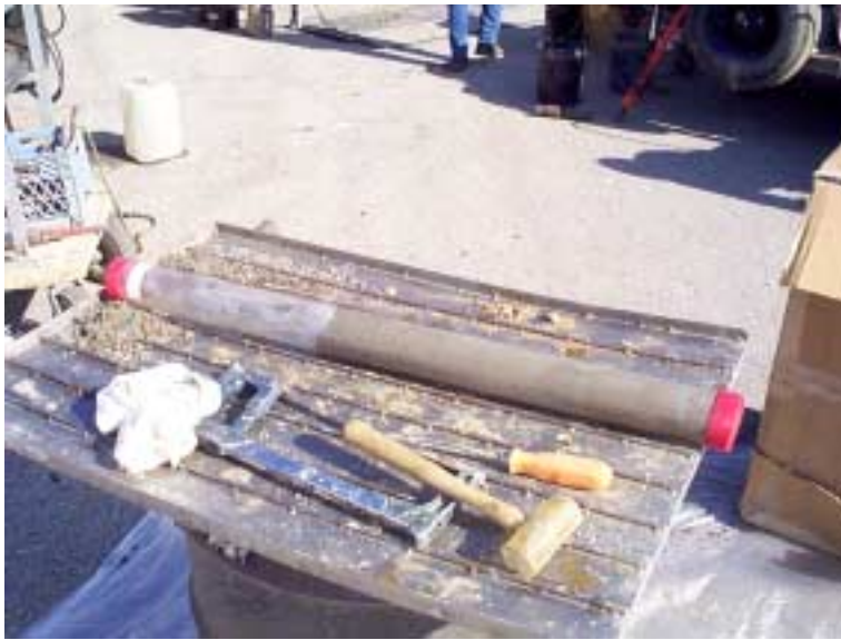
Image 3. Soil sample recovered in an acrylic liner using a Vibracore.
