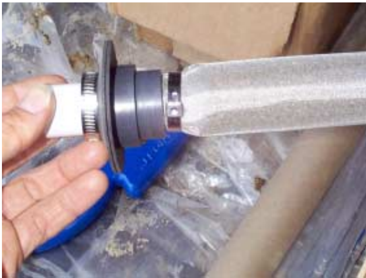
Image 8. Preparation of a \frac{3}{4} -inch prepack direct-push well.
