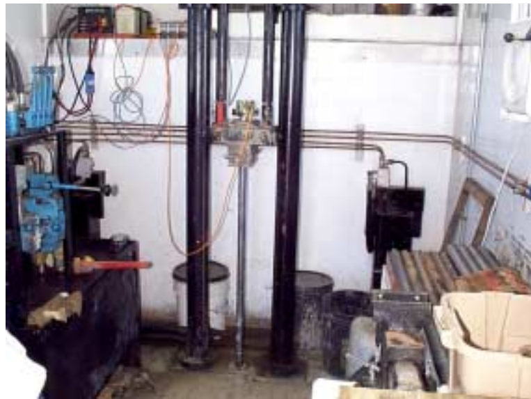
Image 2. Advancement of the wireless piezocone.
