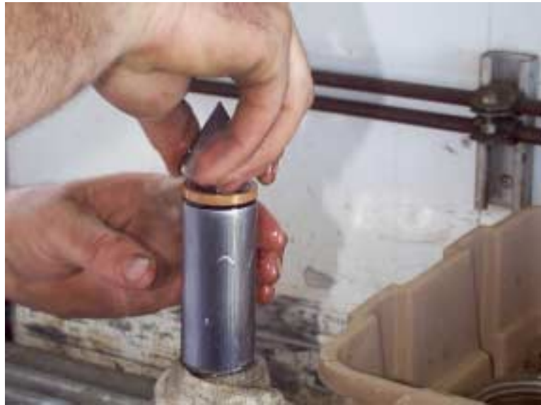
Image 1. Preparation of piezocone probe.
