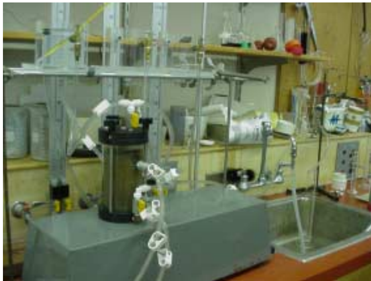
Image 4. Permeability test cell.
