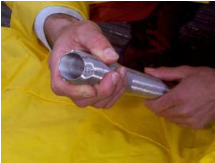
Image 7. Prepack filter for a \frac{3}{4} -inch direct-push well.
