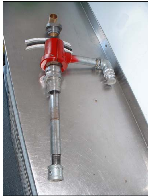
Figure 2-6. EAPS drill/push apparatus
