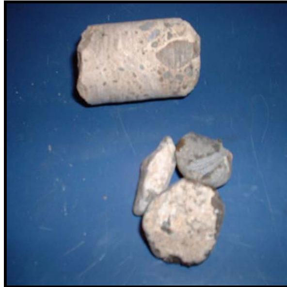
Figure 2-9. Cemented Cold Creek caliche core section sample collected by the core barrel sampler.
