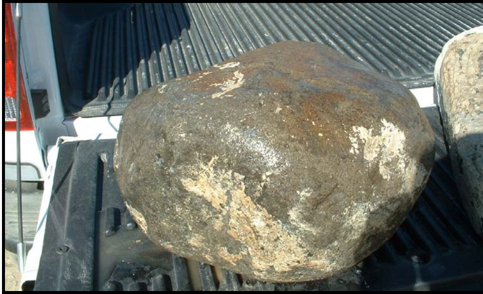
Figure 3-2. Close-up of basaltic cobble from Ringold formation.
