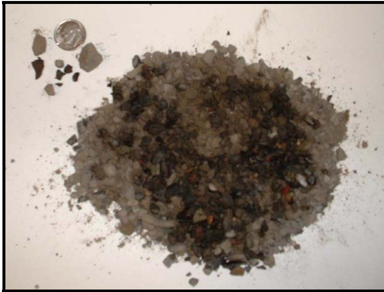
Figure 2-16. Drill cuttings, showing chip size cut primarily basaltic rock.
