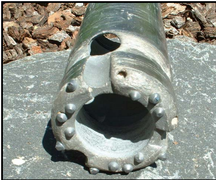
Figure 2-15. Early test prototype, large ring bit showing wear and two missing carbide buttons after drilling through 145-ft. at Hanford.
