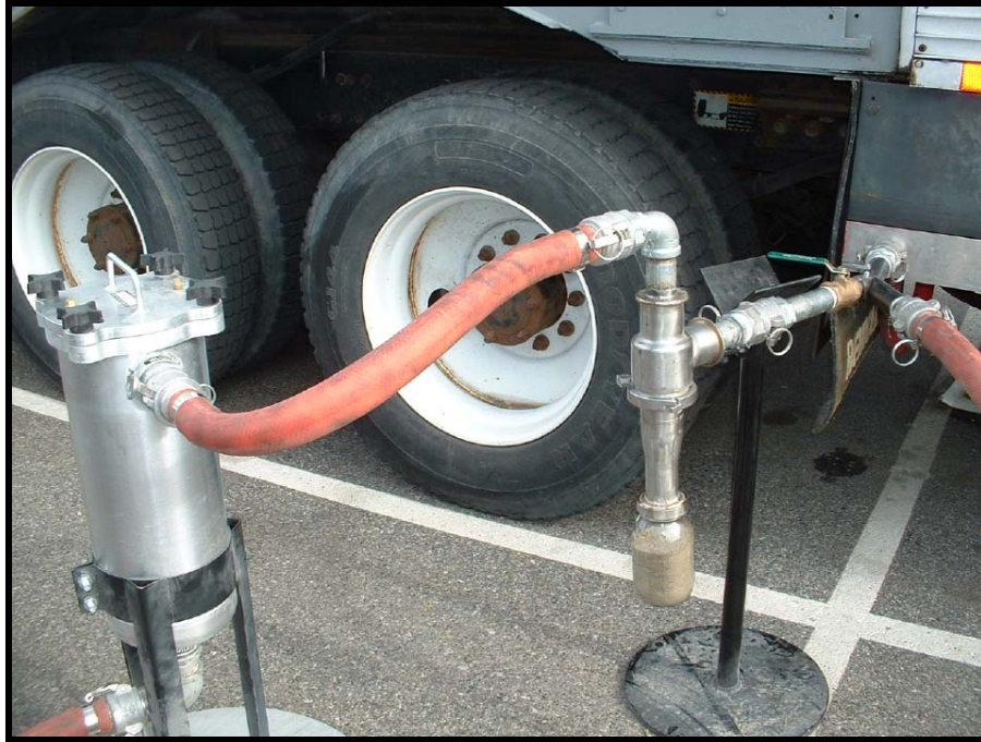
Figure 2-10. Particulate sampler (left side), geological sampler (right side) configured in series.
