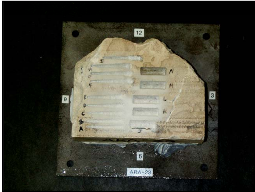
Figure 2-1. Caliche sample ARA-23 showing laser drilled linear tracks (left) and drilled areas (right).
