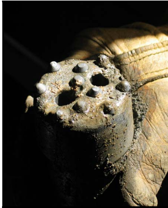
Figure 2-5. Center hammer bit after more than 700 feet of drilling.
