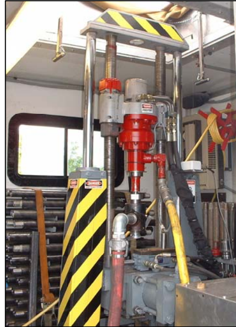
Figure 2-6. EAPS drill/push apparatus
