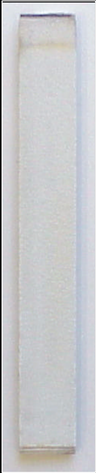
EBC coated CMC run 1000 h in the combustor rig
