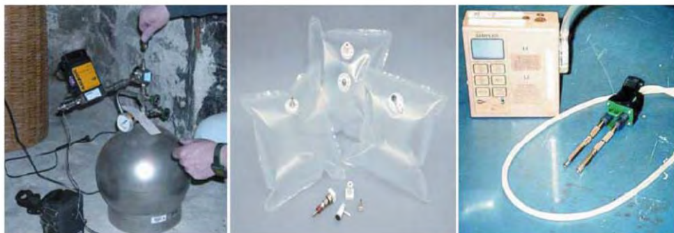
Figure 2. Types of Sampling Equipment (from left to right: Canisters, Tedlar Bags, and Sorbent Tubes) (EPA 2008a)
