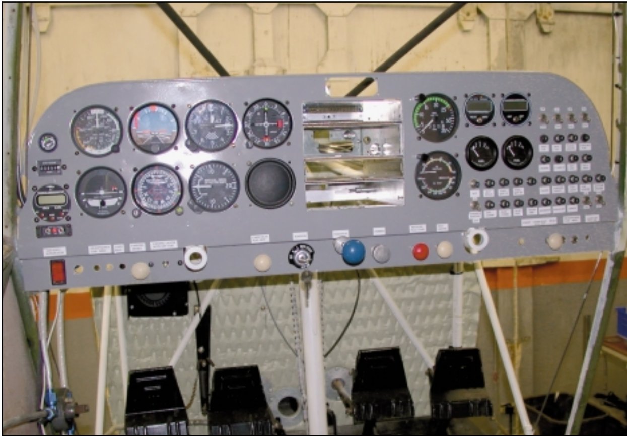
The new panel takes shape. Once the new communications and IFR navigation gear and second course deviation indicator are installed, it is hard to believe this is a 1953 Tripacer.
