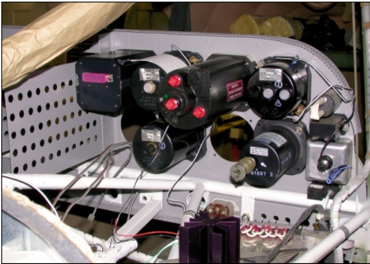
It took four tries to make a custom panel to fit all of these flight instruments into an aircraft almost 50 years old. The challenge was in fitting them around the structural tubing.
