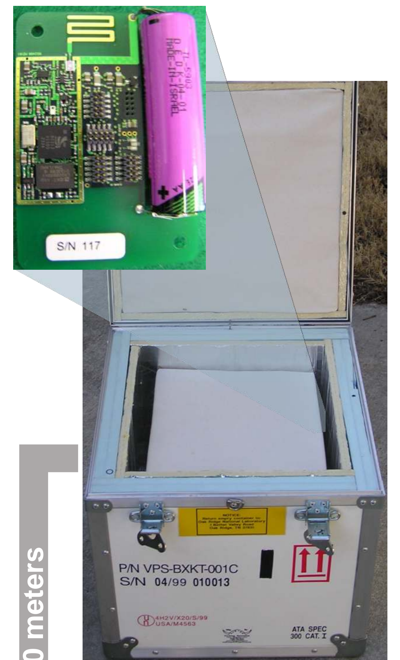
Modified Type A Radioactive Material Shipping Container: Wireless tag embedded in wall
