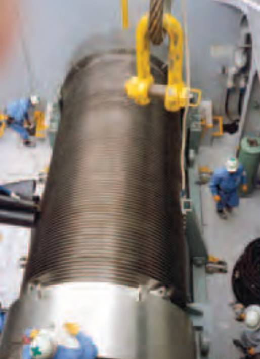
Spent fuel flask being loaded for domestic sea movement in Japan (1992). © IAEA/John Mairs
