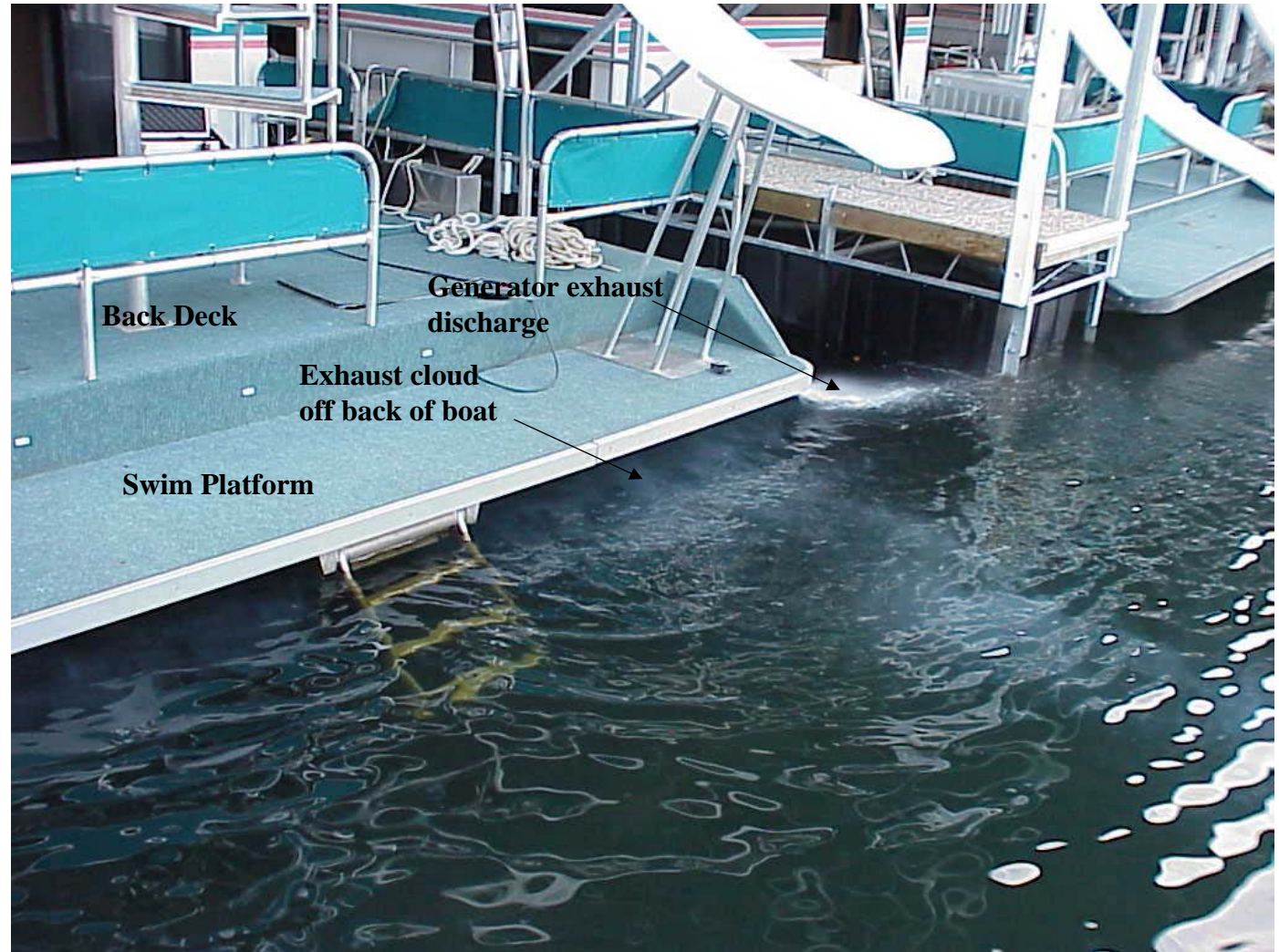
Figure 2. Back View of Navigator boat and generator exhaust discharge.
