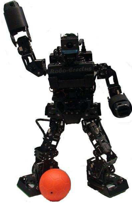
Figure 2. Robo-Erectus Junior, the Latest Generation of the Family Robo-Erectus
