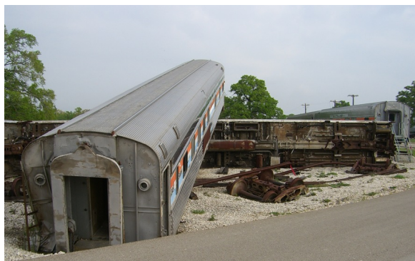
Figure 3: Passenger trains training scenario which simulates the collision and partial derailment of passenger rail cars.
