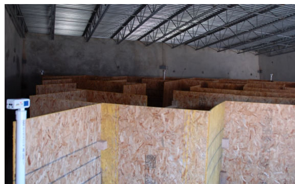
Figure 6: Theater maze test method which tests the ability of a robot to navigate a complex environment without getting lost.
