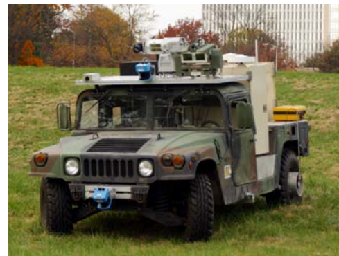
Figure 2: UMS equipped for operating in unstructured environments
