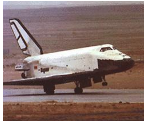
Figure 2: The Soviet Space Shuttle “Buran” touching down automatically upon returning from space in its first and only test flight in 1988.
