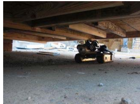
Figure 1: Robot performing mission in confined space
