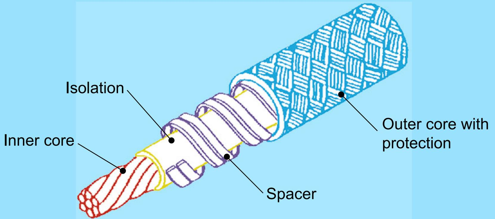
A special sensor cable designed to detect only hydrocarbons while ignoring water is used.
