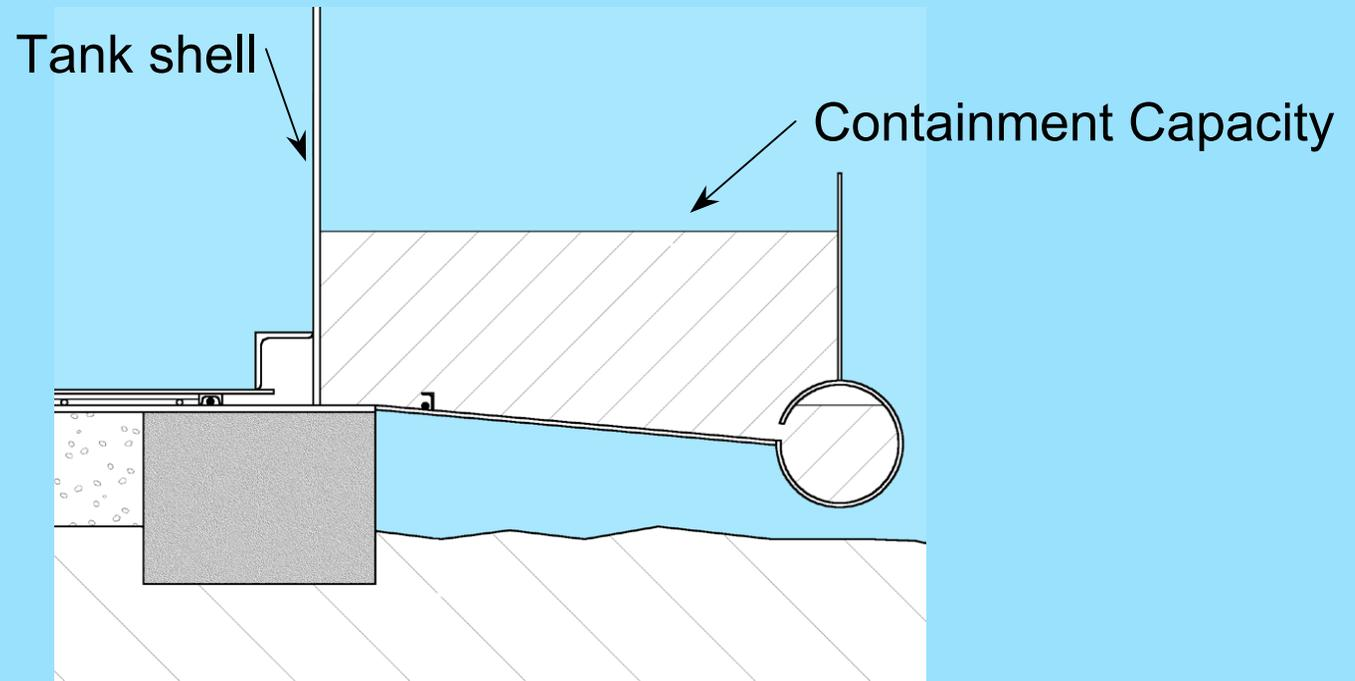
The capacity of the system is designed to contain an amount equal to (or exceeding) the volume of product (worst case scenario) as calculated by the fill valve flow rate relative to the time interval from alarm until the pump is closed or stopped.
