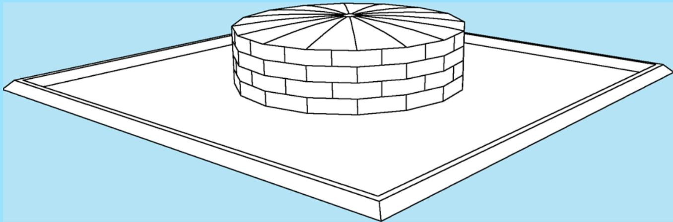
Dike areas must be constructed of materials that will withstand chemical attacks caused by the substance released from the tank.
