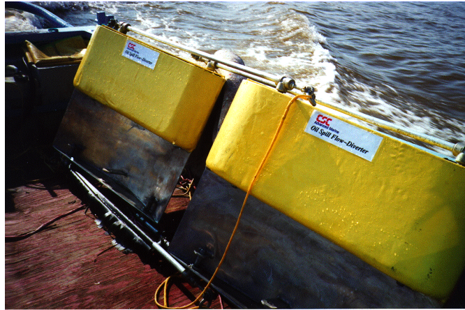
Figure 9. Flow Diverter Catamaran Closed for Quick Transport or Storage
