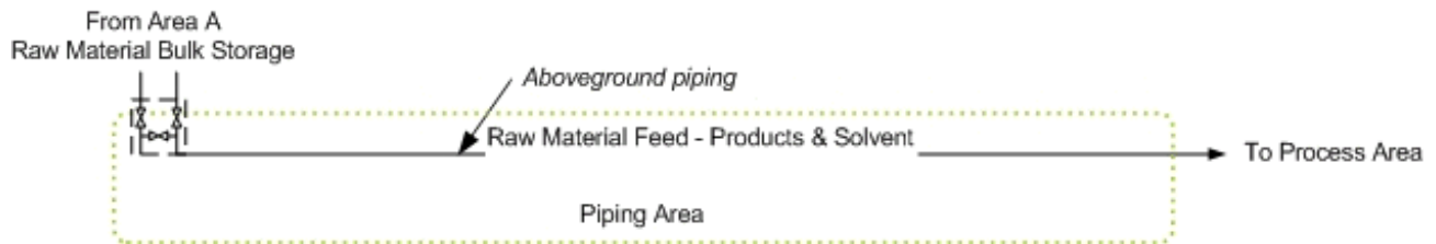
Figure 6-2. Example showing how a complex piping area could be represented in a facility diagram. Note that more detailed diagrams would need to be available at the facility.
