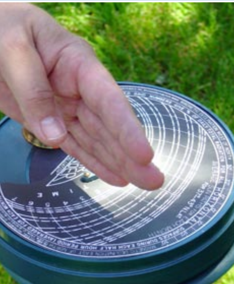
The Solar Pathfinder is used in the field to evaluate and document shading. Photo courtesy of Heidi Steward of PNNL.
