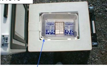
VAXICOOL HAS AN INSIDE DIMENSION OF 14 (LENGTH) BY 10-1/2 (WIDTH) BY 10 (DEPTH) ITS PAYLOAD
