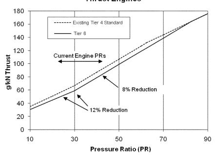
Figure 1: Tier 6 NOx Standards for <u>Higher</u> Thrust Engines
