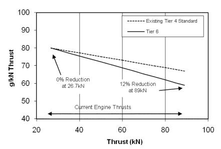
Figure 3: Tier 6 NOx Standards for <u>Lower</u> Thrust Engines At Pressure Ratio 30
